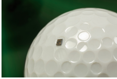
Figure 1.2: The world's smallest ARM-based microcontroller: Kinetis KL03 by Freescale(reproduced from [7]).
