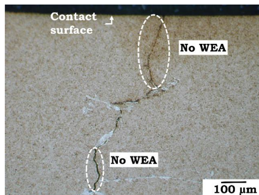
Figure 2.9: LOM image of WEC network where perpendicular to the surface crack appear without WEA [16].
