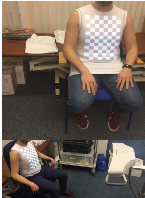
Figure 6-1: SLP projected light grid pattern on participant
