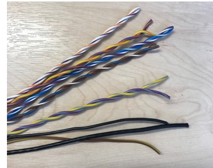
Figure 5.9 – Measured cable bundle; typical wiring from the automotive industry.
