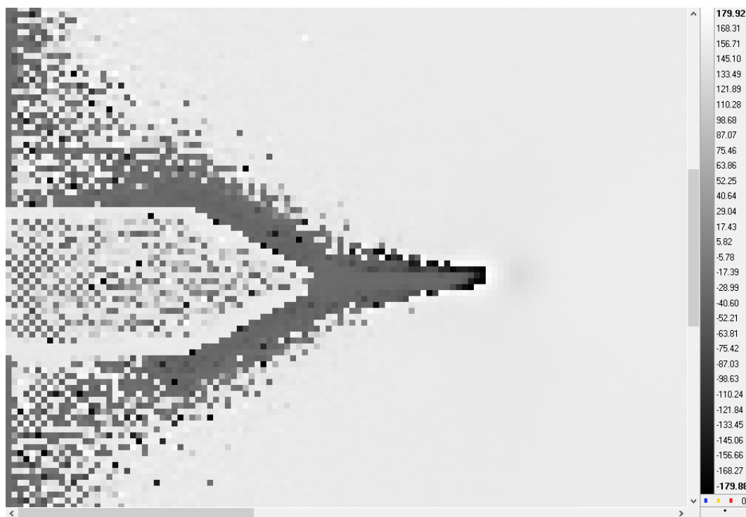
Figure 5.5. Typical photon detector phase image from the specimen loaded at constant load around the specimen crack.
