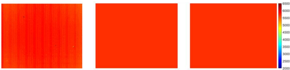
Figure 3.20. Comparison between the photon detector blackbody experiment, average model (centre) and max model (right) at 50 °C.
