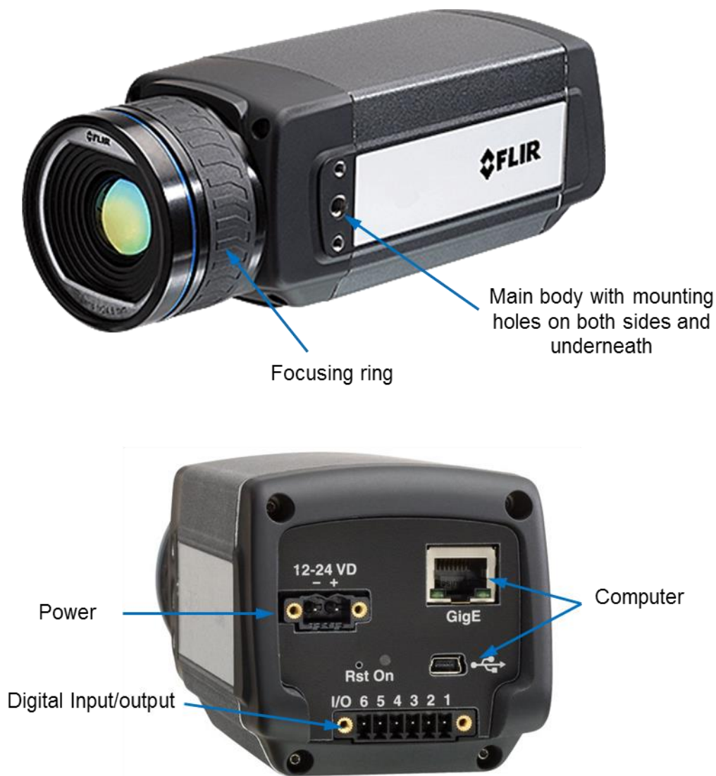
Figure 3.4. A FLIR A655SC Microbolometer [85].
