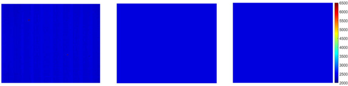
Figure 3.19. Comparison between the photon detector blackbody experiment, average model (centre) and max model (right) at 15 °C.
