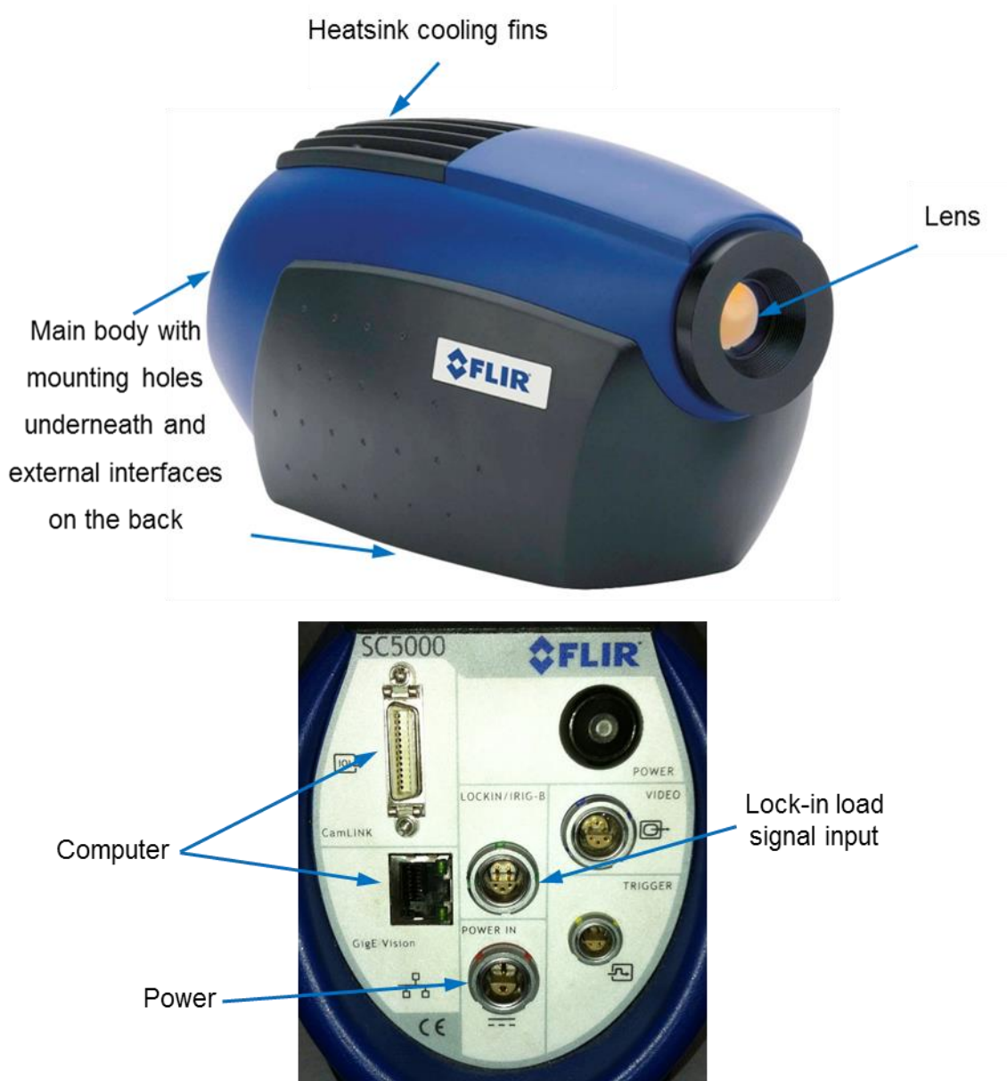
Figure 3.3. A FLIR SC5500 photon detector [82].
