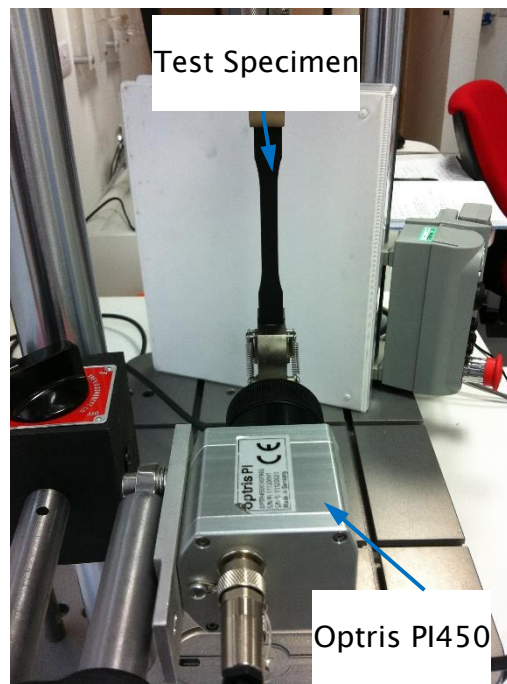
Figure 7.6. Trial set-up for Optris PI450 Microbolometer.
