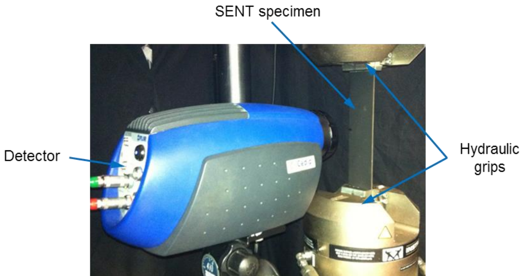
Figure 4.7. SENT specimen test arrangement.
