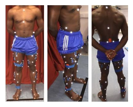
FIG 6.1. MARKER AND SENSOR SETUP FOR LABORATORY BASED MOTION CAPTURE. A total of 48 fluorescent markers of varying sizes were attached to the participant's torso and legs, in order to facilitate the creation of a complex virtual human biomechanical model for the purpose of motion analysis. Additionally, 3 inertial and magnetic sensors were attached to the sacral area, the distal thigh and the distal shank for the purpose of validating a relatively new motion capture method.
