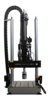
**Fig 3.2. INSTRON D8874 – AXIAL – TORSION FATIGUE TESTING SYSTEM.** The Instron D 8874 is a bi-axial servo hydraulic testing system, often used in Biomedical and component testing applications. The Instron is equipped with a Linear Variable Differential Transformer and a Rotational Variable Differential Transformer, which guarantee translational and rotational measurements to an accuracy of up to  $\pm 1-2^{\circ}$ .
