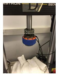
Fig 3.4. LABORATORY SETUP FOR SENSOR ACCURACY TEST.
