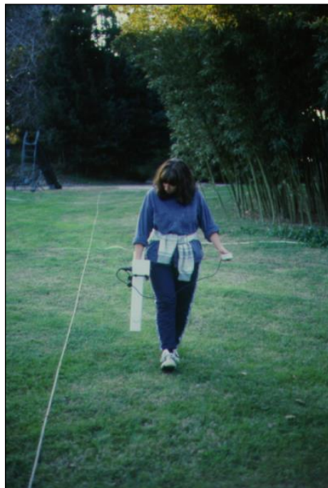
Figure 5.11 Magnetometry being conducted at Portus in 1998 using a Geoscan Research FM36 fluxgate gradiometer (photo: K. Strutt)
