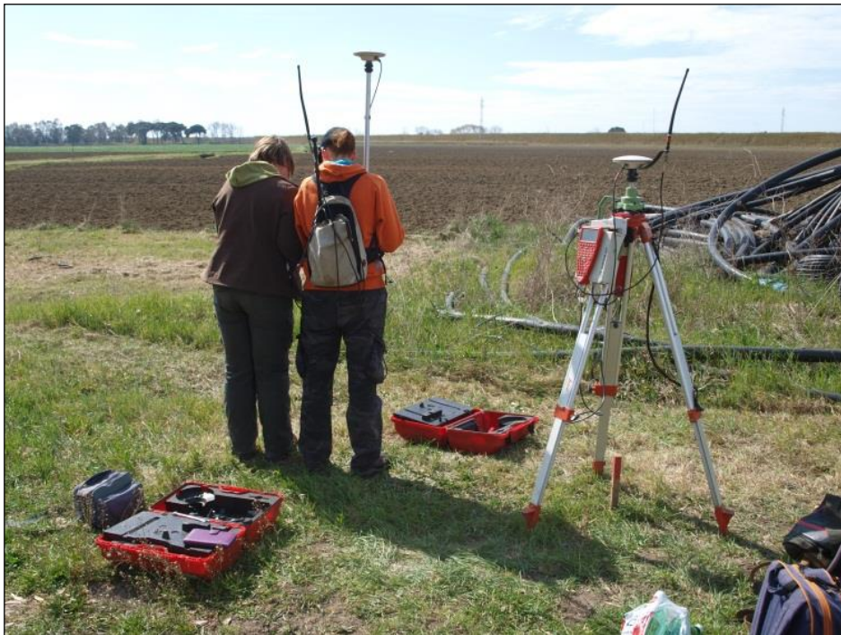
Figure 5.10 Use of RTK GPS in the field to the east of Ostia Antica (photo: K. Strutt)
