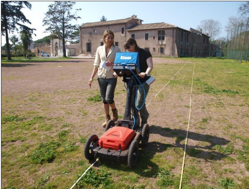
Figure 5.14 Ground Penetrating Radar (GPR) survey being conducted close to the Episcopio at Portus, using a GSSI 400MHz antenna with SIR-3000 console and cart (photo: K. Strutt)
