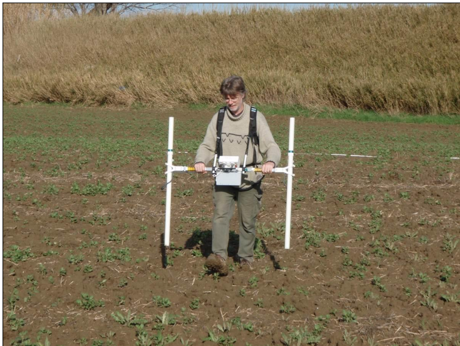
Figure 5.13 Magnetometer survey being conducted with a Bartington Instruments Grad 601 fluxgate gradiometer (photo: K. Strutt)
