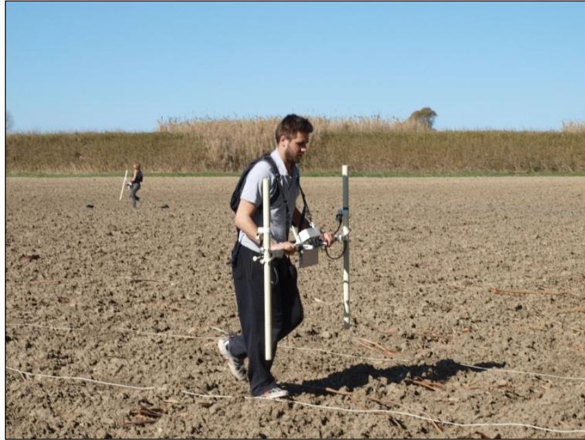
Figure 5.12 Magnetometer survey on the Isola Sacra, close to the modern course of the Tiber, using Bartington Grad 601 fluxgate gradiometers (photo: K. Strutt)
