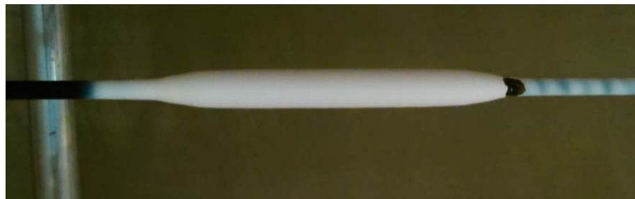
Image 33. Crack-free germania deposition.
