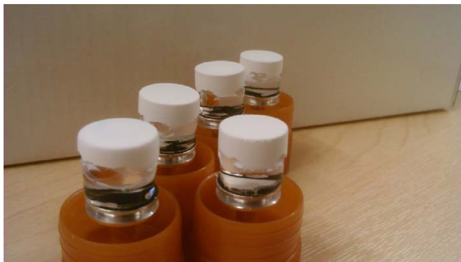
Image 11. Deposition samples for SEM and XRD characterisations.
