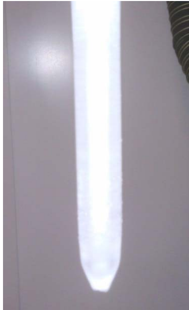
Image 40. Preform OVD0025 after the consolidation process.
