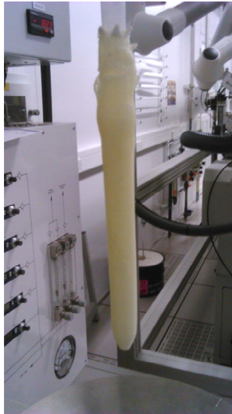
Image 49. Preform OVD0023 after the consolidation process.
