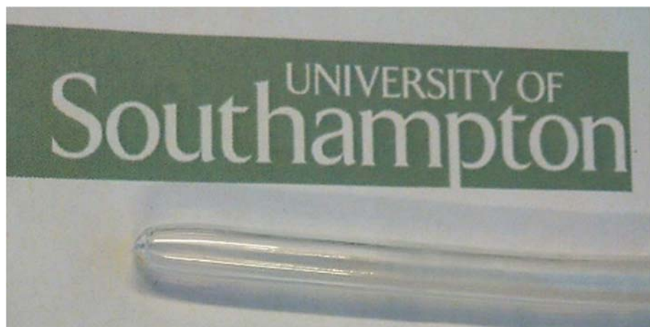
Image 36. Transparent and defect free 100% GeO 2 preform
