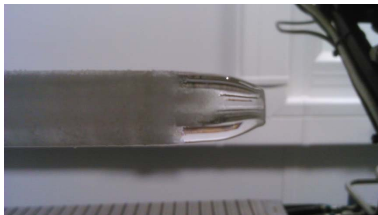
Image 41. Preform OVD0025 made transparent after heating the tip.
