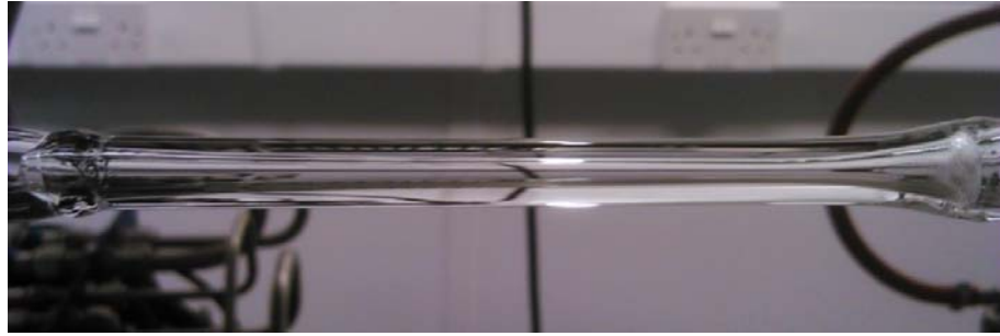
Image 47. Preform OVD0026 after the collapsing process.
