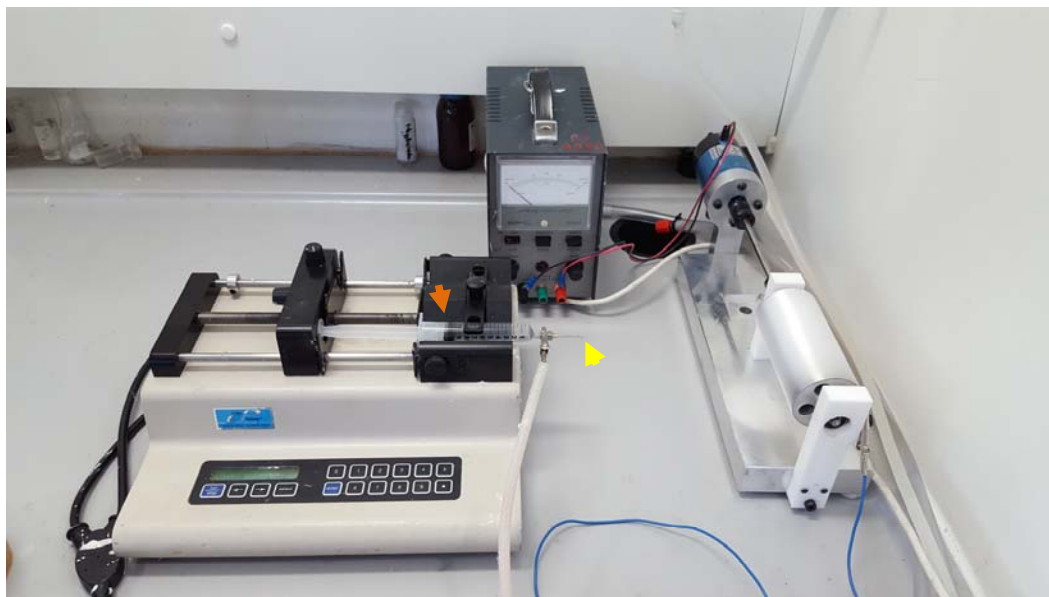
Figure 20: Picture of the electrospinning set-up, showing: (left) the syringe pump with syringe & needle clamped in place (orange arrow); (centre) the voltage generator; and (right) the rotating collector where the electrospun membranes are generated. The needle is connected to the voltage generator and the polymer is driven through the needle (yellow arrow) and spins into a fibrous mat.
