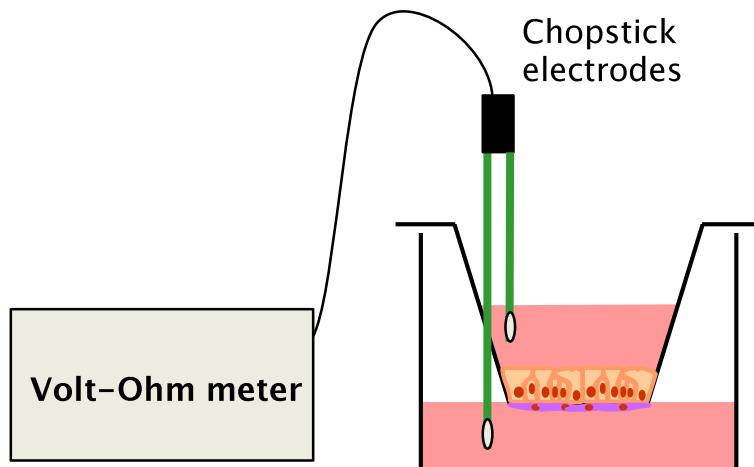
Figure 2.7.1-1 Measurement of TER using chopstick electrodes and a Volt-Ohm meter.
