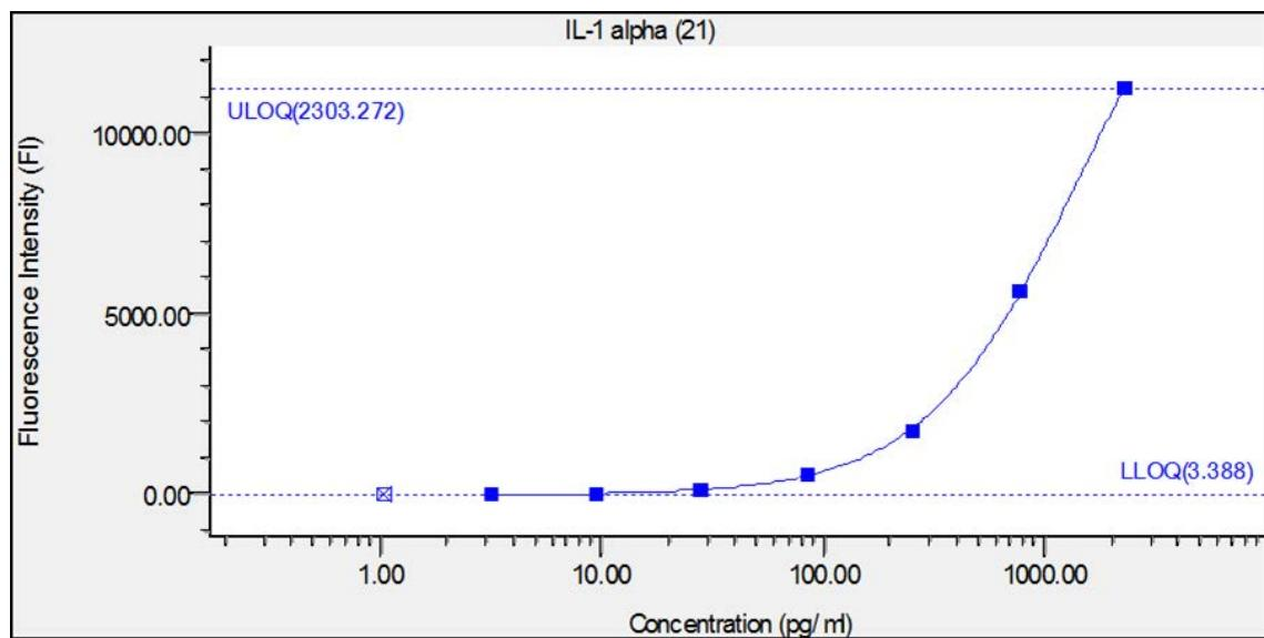
Figure 2.11.2-2 Typical Luminex® screening assay standard curve generated using the Bio-Plex software.
