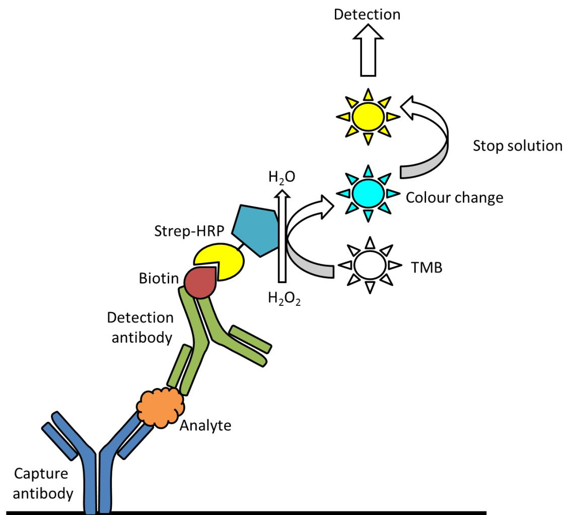
Figure 2.11.1-1 Overview of the sandwich ELISA for the detection of analytes. If antibody-analyte-antibody-strep-HRP complexes form, TMB is converted to a coloured product. Thus the colour change indicates the presence of the antigen of interest [201, 202].
