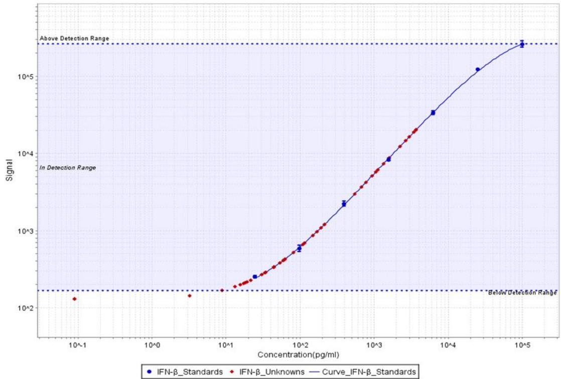
Figure 2.11.3-2 MSD® human IFN-β assay standard curve generated using the SECTOR Imager 6000 software.
