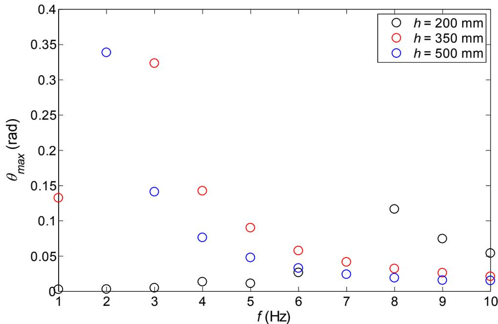
**Figure 7.** Maximum angular displacement versus excitation frequency for blocks with  $F_{c0} = 0$  kN and different heights.
