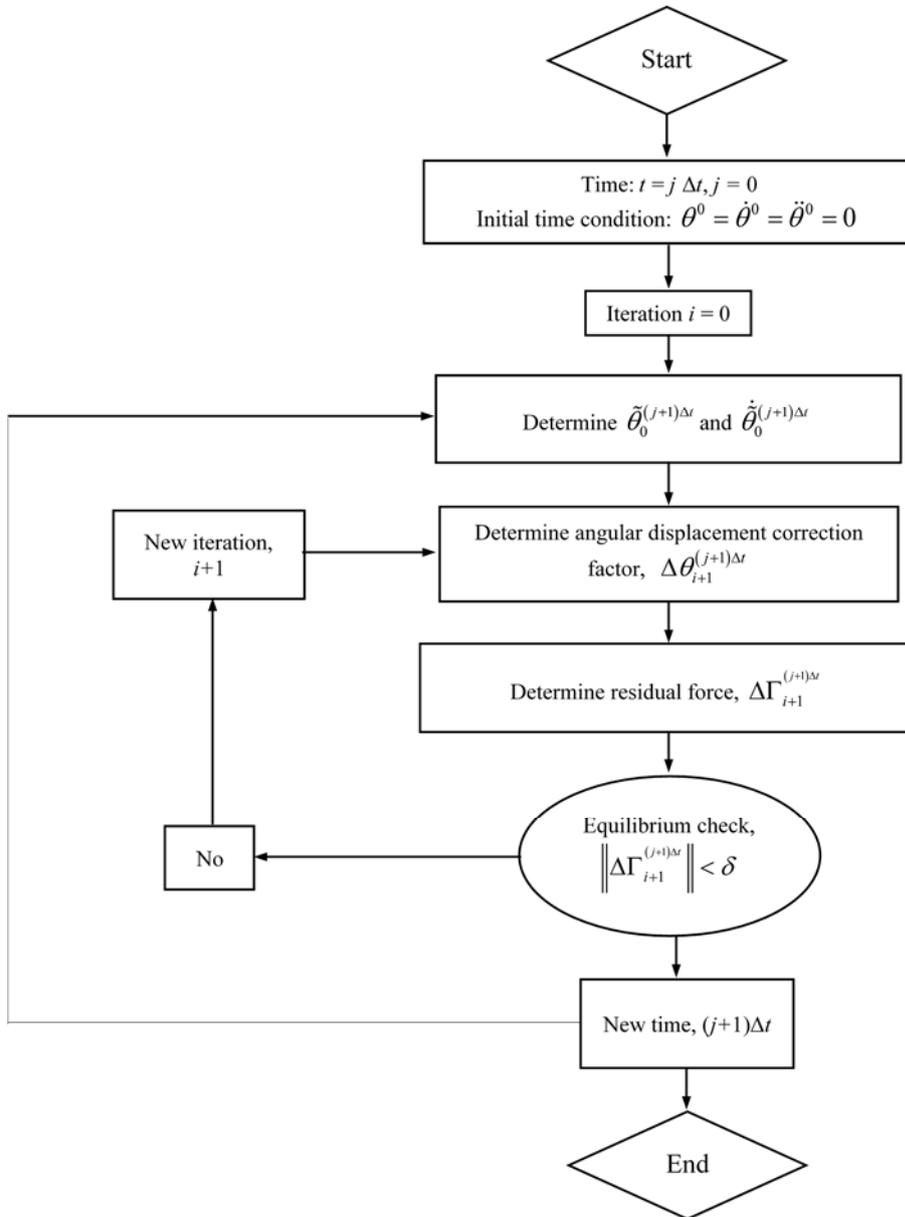
**Figure 3.** Algorithm used for numerical analysis of the nonlinear rocking equation of motion.
