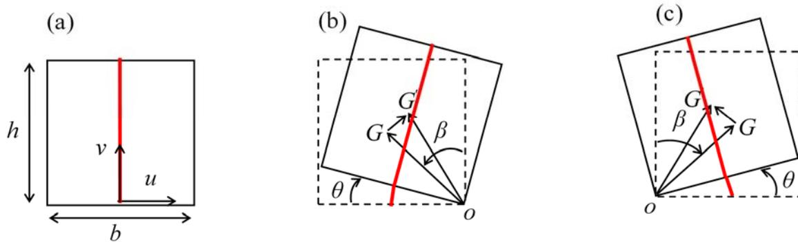
**Figure 1.** (a) Positive rocking positive rocking ( $\theta > 0$ ) and  $\alpha < 0$ , and (b) negative rocking ( $\theta < 0$ ) and  $\alpha > 0$ .
