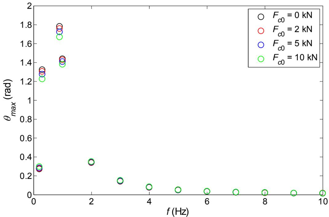
**Figure 6.** Maximum angular displacement versus excitation frequency for blocks with  $h = 500$  m and different initial pre-tensioning forces.
