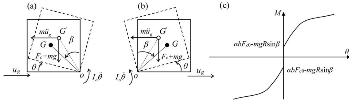
**Figure 2.** Free-body diagram of a single block: (a)  $\theta > 0$ , and (b)  $\theta < 0$ , and (c) moment-rotation relationship of a single block.
