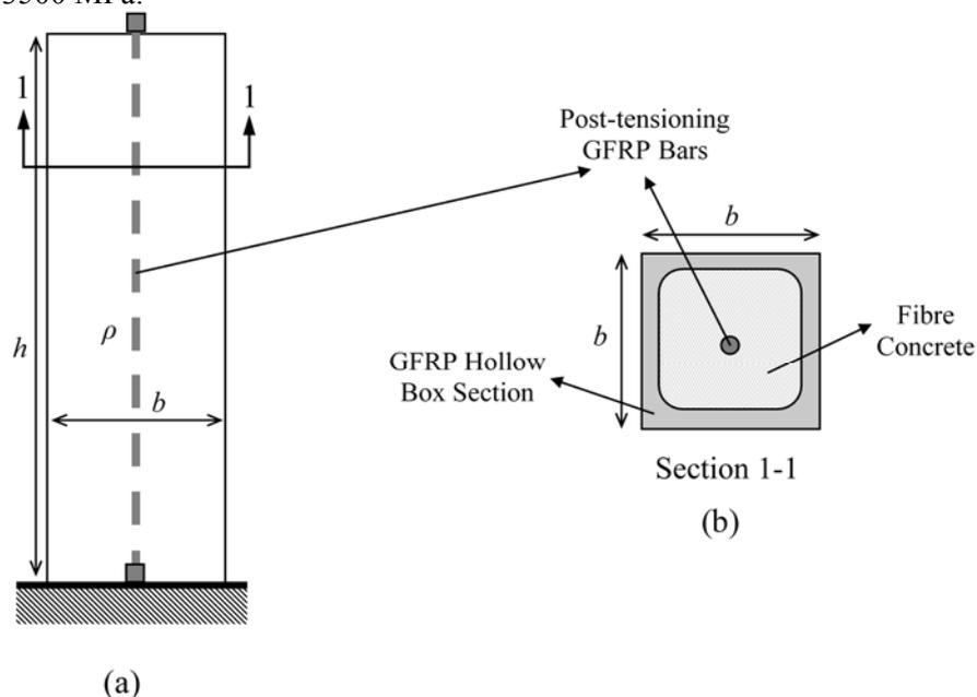
**Figure 4.** (a) Composite pre-tensioned block, and (b) block section details.
