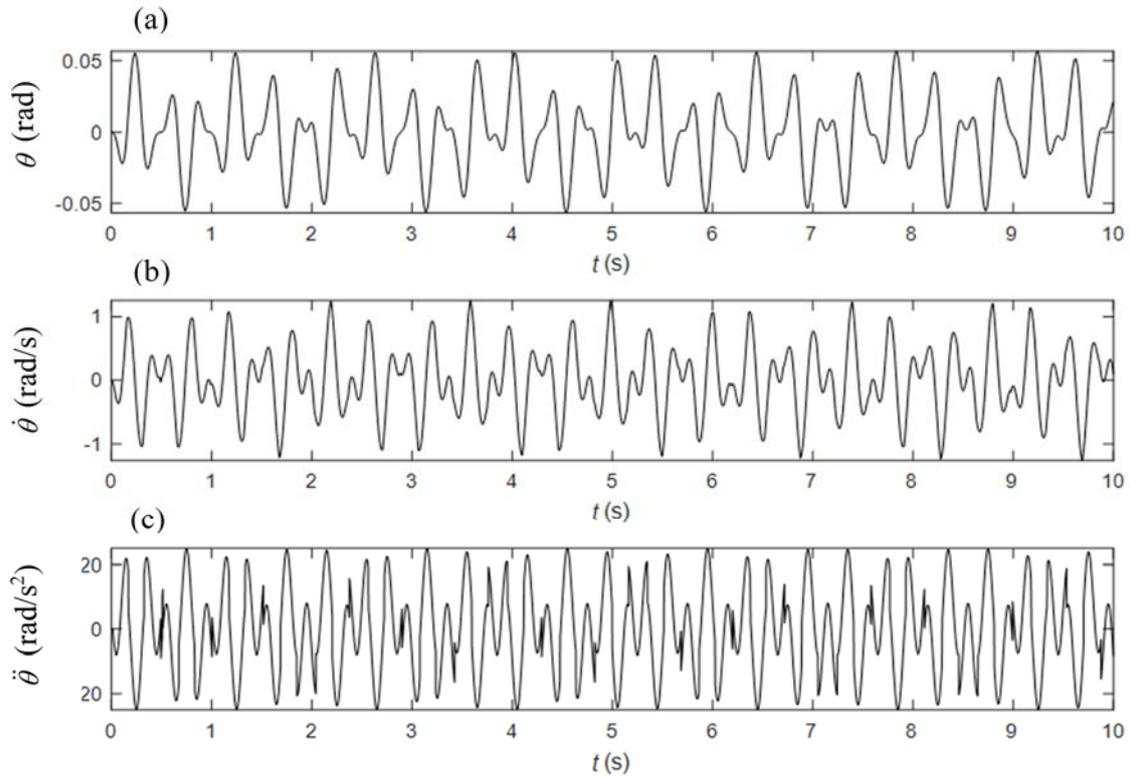
**Figure 5.** Time-history analysis: (a) angular displacement, (b) angular acceleration, and (c) angular acceleration.
