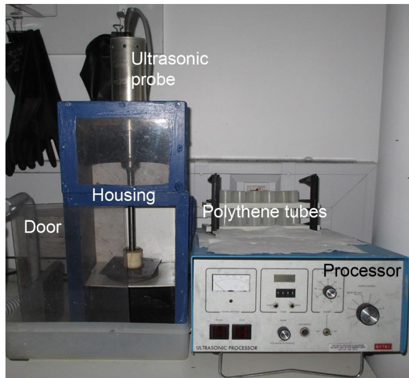
Figure 45. Photograph of the ultrasonic probe used to remove extraneous AOM from palynomorph samples that contained scolecodonts.
