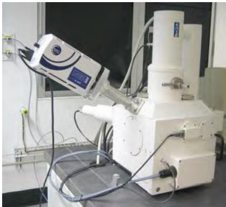
Figure 40. Photograph of the Carl Zeiss Leo 1450VP SEM with Oxford Instruments Energy Dispersive Spectrometer at the University of Southampton. From https://cdn.southampton.ac.uk .
