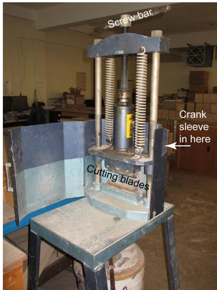
Figure 32. Photograph of the pneumatic jack used to split hard sediments.
