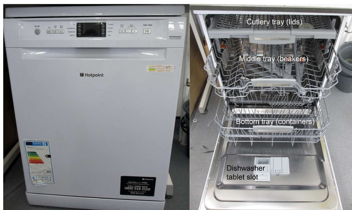
Figure 153. Photographs of the dishwasher used to clean the containers, lids and beakers used in palynological processing – door closed (left hand side) and door open (right hand side).
