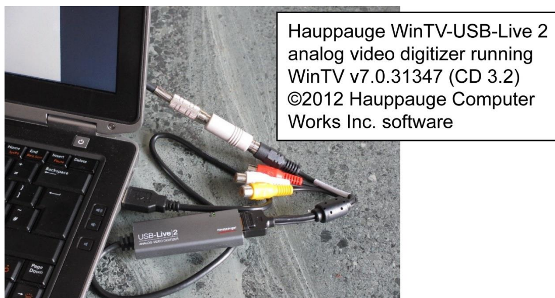
Figure 37. Photograph of the analogue video digitizer to output digital images from analogue signal.
