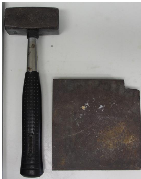
Figure 136. Hammer (Draper 1 lb on left-hand side) and metal block (right-hand side) used to crush rock samples to pea-sized chips before processing.
