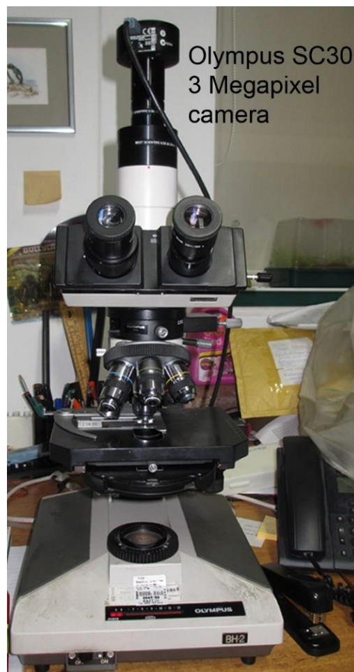
Figure 34. Photograph of the Olympus BH-313 light microscope (number: 210685) with an Olympus SC30 3 Megapixel camera mounted on a trinocular head.
