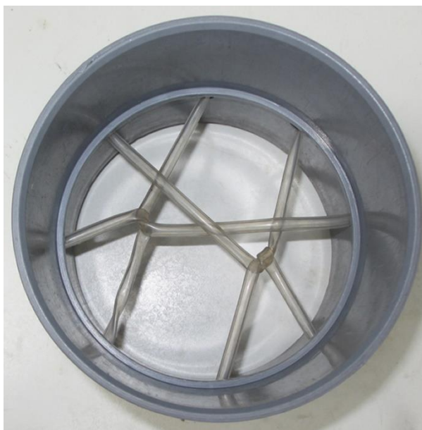
Figure 150. Photograph of the elasticated grey stand used to house the medium sieve to enable it to drain while setting the next sample to boil.
