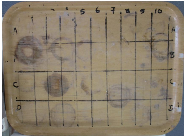
Figure 162. Photograph of a slide tray with numbered segments to place coverslips containing palynological samples during drying before being made into permanent slides.
