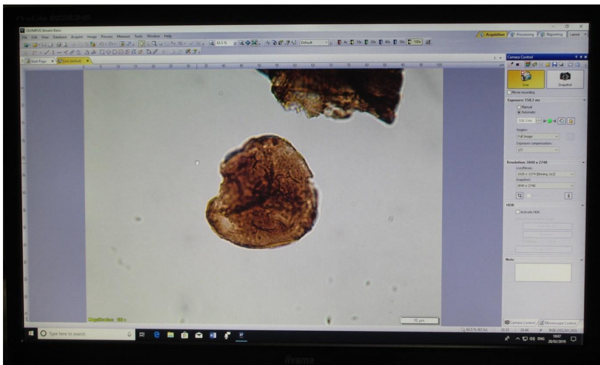
Figure 35. Photograph of the PC monitor with the Olympus Stream (Basic) photomicroscopy software loaded showing a live image of a Plicatispora scolecophora miospore at x100 on the Olympus BH-313 light microscope in Figure 34.
