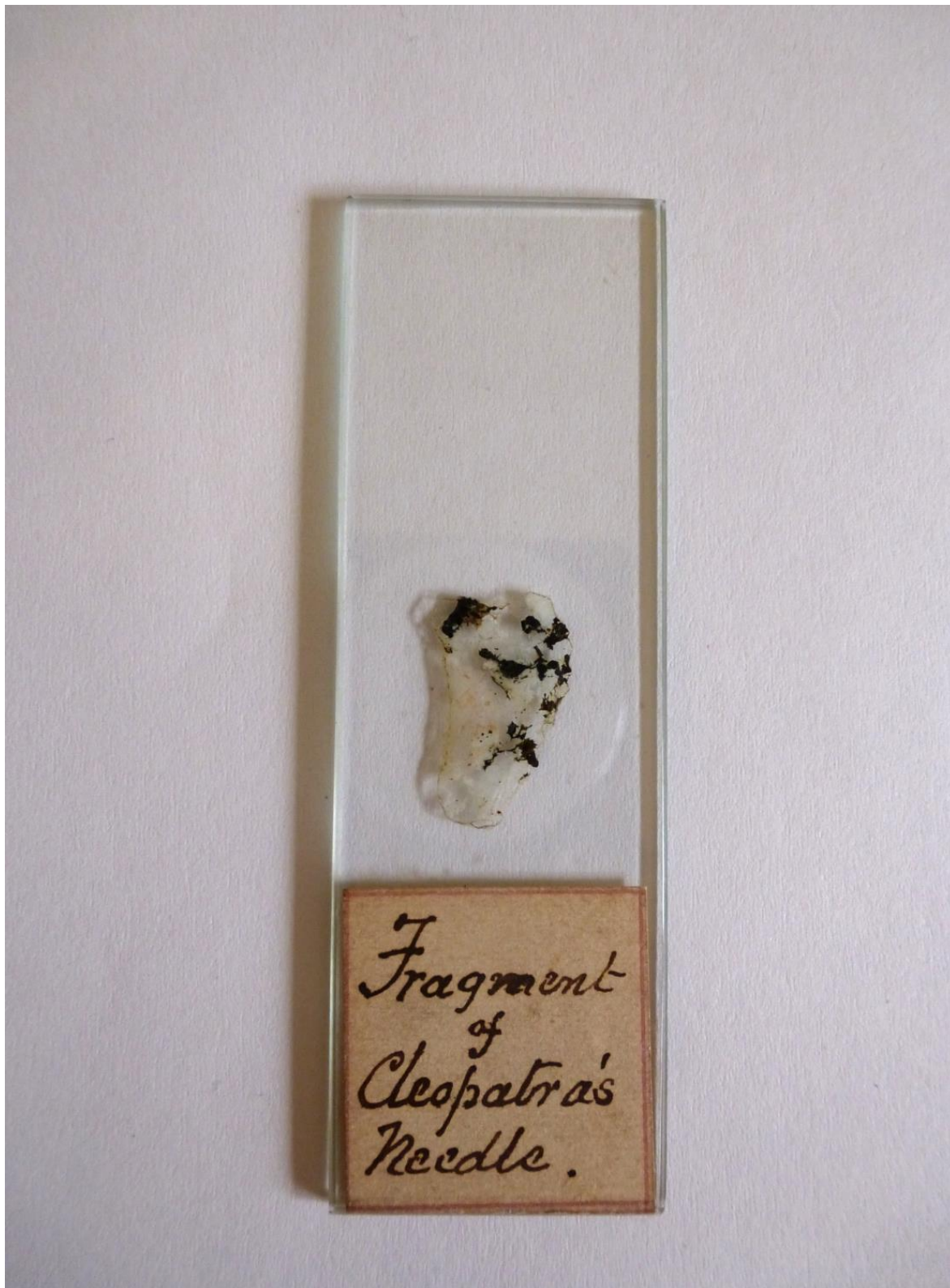
Figure 22 - A professionally prepared microscope slide of granite from Cleopatra's Needle.
