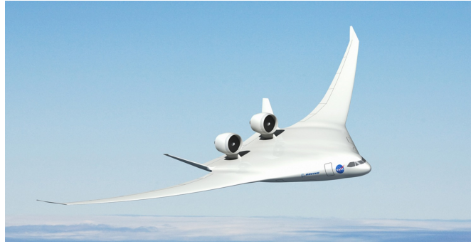
Figure 1.3: BWB concept proposed by Boeing/NASA.
