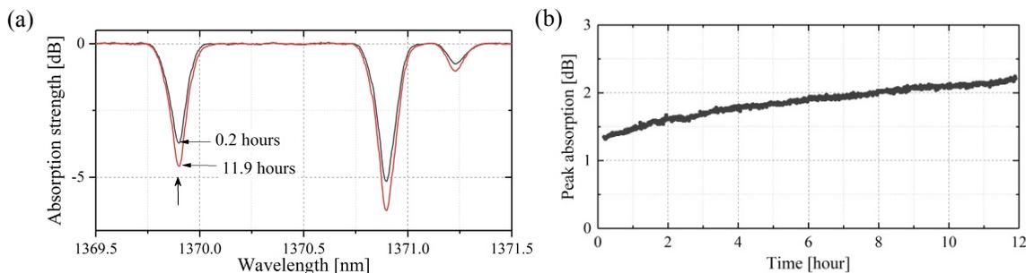
Fig. 2: (a) Evolution of spectral absorption of water vapour in 35 m of PBGF-A with time. The arrowed line is at 1369.85 nm. (b) Ingress of water vapour in PBGF-A; the sample was open to the atmosphere for 12 hours. The measurement time was started when the first fibre end was cleaved.
