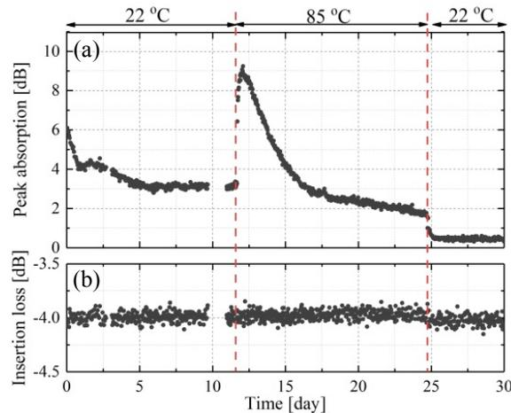
Fig 4: Variation of (a) water vapour absorption strength and (b) insertion loss at 1550 nm recorded at 2 nm resolution in PBGF-D with high time resolution.
