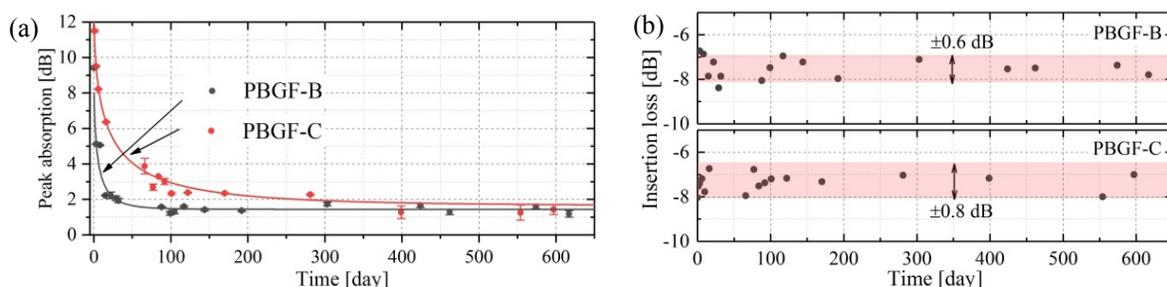
Fig 3: (a) Evolution of water vapour absorption strength with respect to time; black circle: PBGF-B at 1369.85 nm, red circle: PBGF-C at 1399.65 nm. (b) Insertion loss at 1550 nm at 10 nm resolution.
