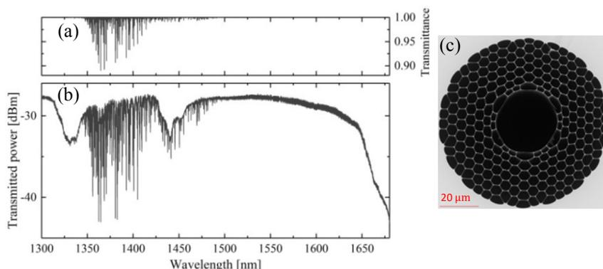
Fig. 1: (a) Transmittance of water vapour from HITRAN database (1 ppm, 1 km, 0.05 nm filter) (b) transmitted spectra recorded at 0.05 nm resolution and (c) scanning electron micrograph of PBGF-A (55 m).
