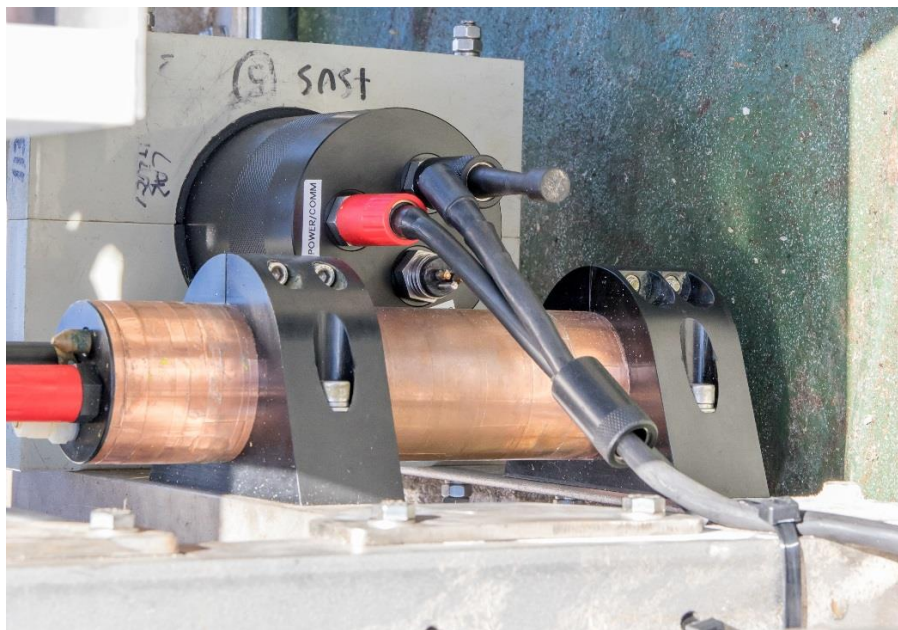
The Wetlabs FLNTSUB with copper and measurement window facing out of the frame (shown towards deck due to frame placement when photograph taken).
