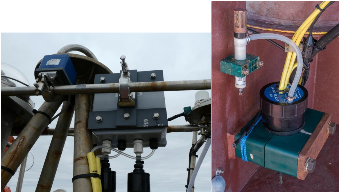
Pro-CO 2 atmospheric unit showing pump and Pro-CO 2 unit on the keel and atmospheric CO 2 unit attached to the top of the buoy.
