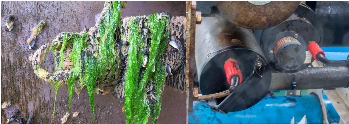
SeaFET copper guards (left SN105 on the buoy, right SN111 on the frame)
