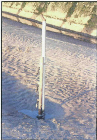
Figure 4-2: Offshore Tell-Tail scour monitor at Blackpool (from HR Wallingford, 2005)
