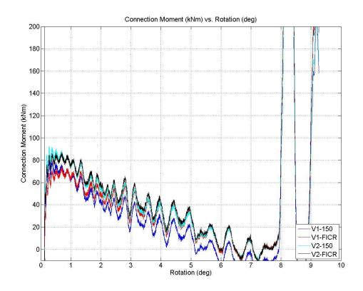
Figure B 54: T8 - Connection moment (kNm) vs. rotation (degrees)
