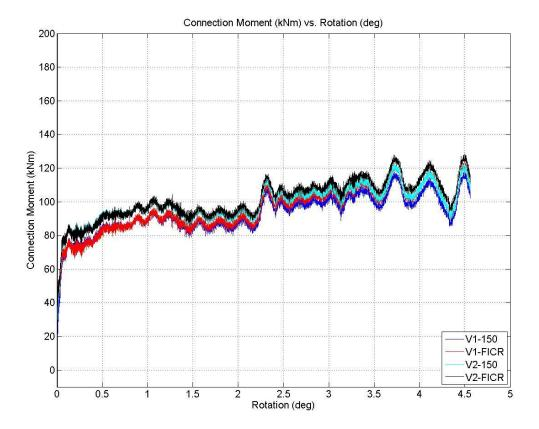
Figure B 28: T4 - Connection moment (kNm) vs. Net rotation (degrees); The four curves represent four versions of the same equation; They give similar values; Only one version of the equation was chosen to be compared with modelling results.
