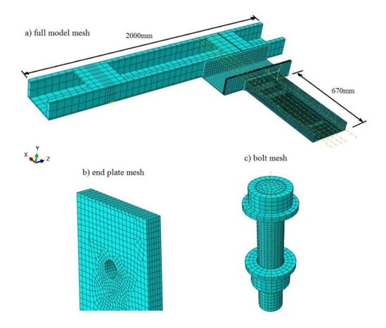
Figure 5.2: Finite element model mesh
