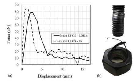
Figure 3.11: Grade 8.8 with one nut (a) force versus displacement and (b) thread stripping
