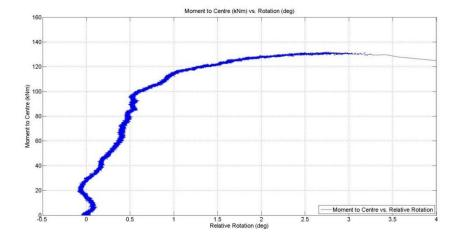
Figure B 13: T6 - Moment to Centre (kNm) vs. Net Rotation (degrees)
