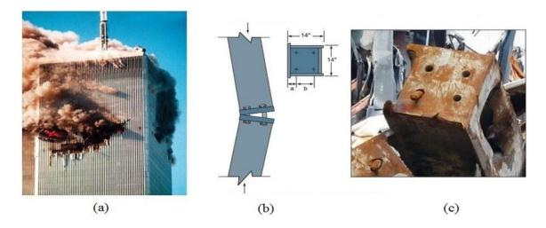
Figure 1.3: (a) Staggered failure pattern where column splices were located, (b) failure mechanism of column and (c) failed connection showing failed bolt (FEMA 2002)
