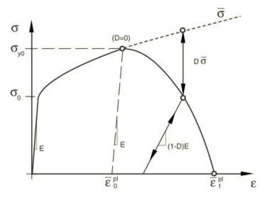
Figure 4.3: Stress-strain curve with progressive damage (Simulia 2015b)
