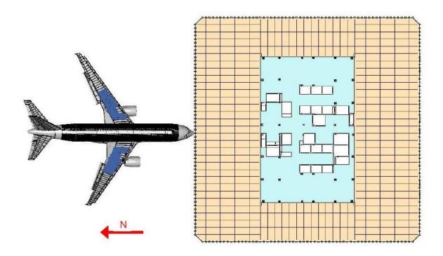
Figure 1.5: Top view of the WTC 1 global impact model (NIST NCSTAR 1 2005)
