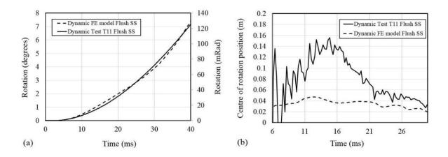
Figure 5.10: (a) Rotation versus time and (b) ICR versus time, note changes are small in comparison to lever arm
