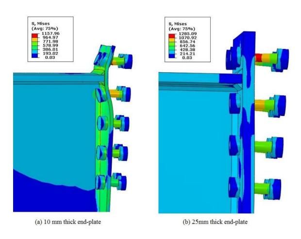
Figure 6.6: Close-up of extended end-plate connection stress plots
