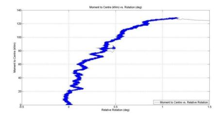
Figure B 4: T1 - Moment to Centre (kNm) vs. Net Rotation (degrees)
