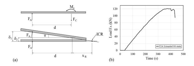
Figure 3.24: Quasi-static loading scenario: (a) free body diagram and (b) test T2A load versus time
