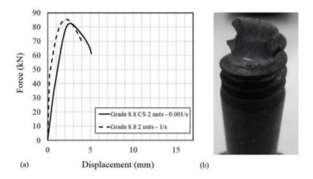
Figure 3.12: Grade 8.8 with two nuts (a) force versus displacement and (b) fracture surface
