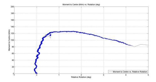
Figure B 8: T2 - Moment to Centre (kNm) vs. Net Rotation (degrees)
