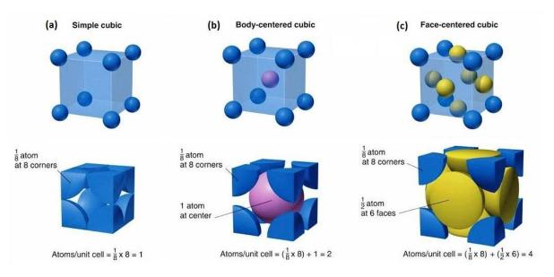
Figure 2.27: Comparison between BCC and FCC crystal structures (Kyawthetlatt 2013)
