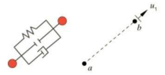
Figure 4.5: Conceptual representation of connector element (Simulia 2015b)
