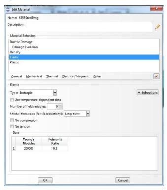
Figure C 1: Defining elastic behaviour of S355 steel
