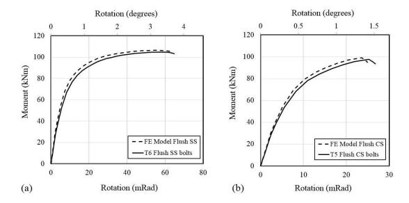
Figure 5.7: Moment versus rotation graphs for flush connections tests and models
