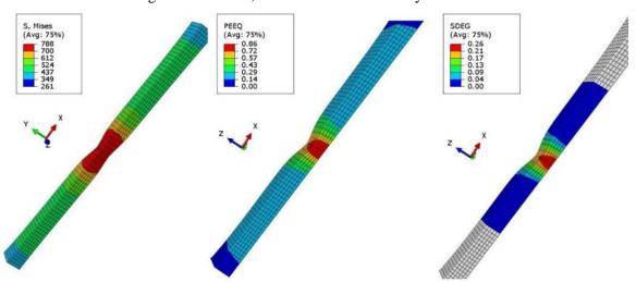
Figure 4.10: Contour plots of Von Mises stresses (S, Mises), equivalent plastic strain (PEEQ) and scalar stiffness degradation (SDEG) at a total displacement of 19.66mm, step time 536s, just before fracture
