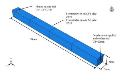
Figure 4.9: Model, dimensions and boundary conditions
