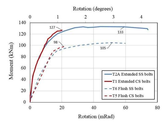
Figure 3.27: Moment versus rotation for quasi-static tests
