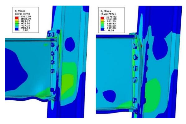
Figure 6.5: Von Mises contour plots for the two types of connections with 20mm thick plates and stainless steel bolts
