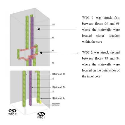
Figure 1.4: Location and orientation of the three stairwells (NIST NCSTAR 1 2005)
