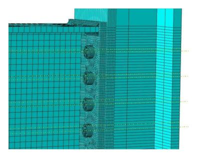
Figure 6.4: Detail illustrating mesh refinement at contact region
