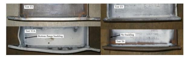
Figure 3.28: Plate deformation with carbon steel (top) and stainless steel bolts (bottom) for quasistatic tests
