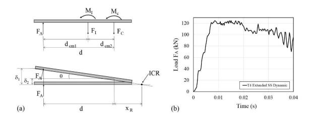
Figure 3.25: Dynamic loading scenario: (a) free body diagram and (b) test T4 load versus time
