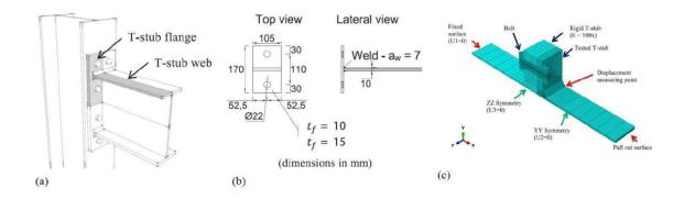
Figure 2.21: (a) T-stub fragment from joint (b) T-stub geometry (c) T-stub numerical model in ABAQUS (Ribeiro, Santiago, Rigueiro, et al. 2015)
