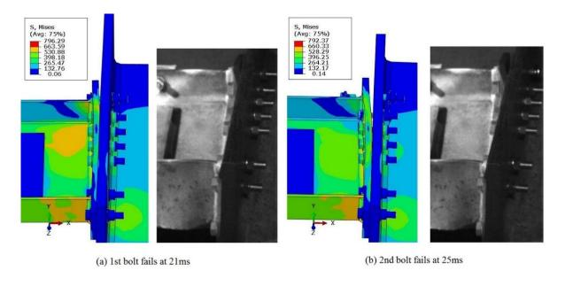
Figure 5.17: 1st bolt fails at 21ms and 2nd bolt fails at 25ms
