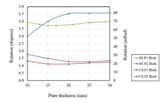
Figure 6.10: Rotation versus plate thickness for flush end-plate connection models
