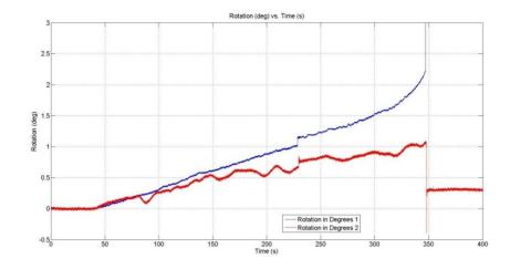
Figure B 3: T1 - Rotation (deg) vs. time (s) of "flying column" (blue) and angle supports (red)
