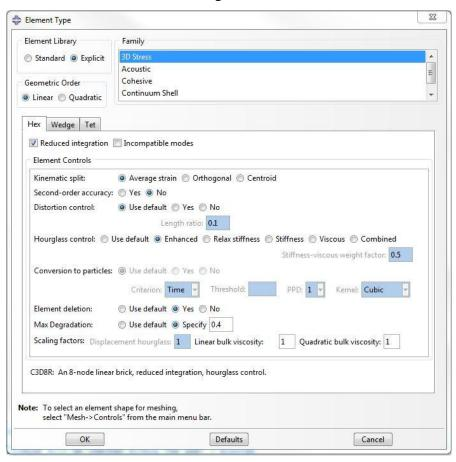
Figure C 9: Defining element type for stainless steel
