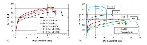
Figure 2.23: Force vs. displacement curves for (a) different applications times and (b) different end-plate thickness of T-stub
