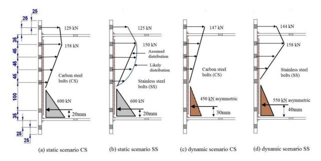
Figure 3.33: Force distribution in static and dynamic loading scenarios
