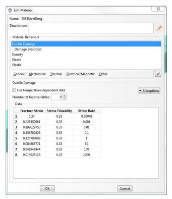
Figure C 3: Defining fracture strain for S355 steel
