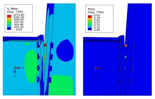
(b) equivalent stresses and plastic strains for 25mm thick flush end-plate
