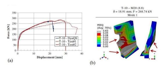
Figure 2.22: (a) Results for quasi-static case and (b) plastic strains and development of two plastic hinges (Ribeiro, Santiago, Rigueiro, et al. 2015)
