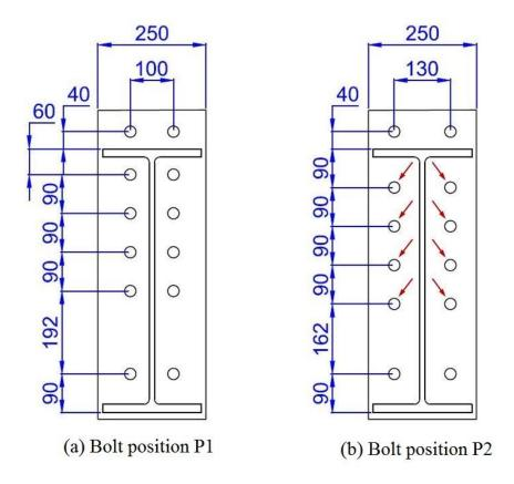
Figure 6.2: Position of bolt holes for the extended plate connection
