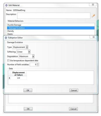
Figure C 4: Defining damage evolution for S355 steel
