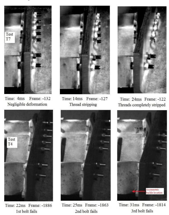
Figure 3.29: Frames captured after commencement of dynamic loading for carbon steel bolted connection (top row) and stainless steel bolted connection (bottom row)
