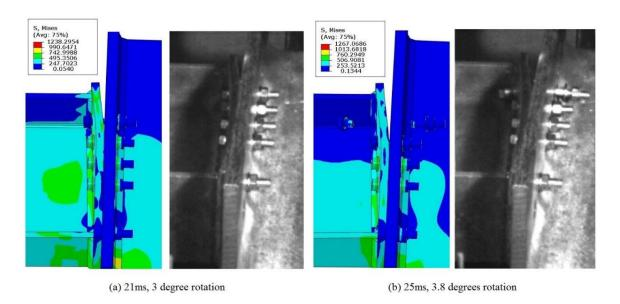
Figure 5.12: 1st and 2nd bolts fails at 21ms and 25ms, predicted and experimental results
