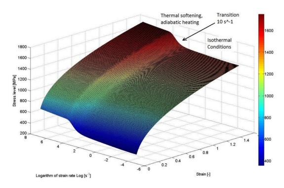
Figure 2.29: Analytical predictions of the constitutive description within wide ranges of strain rates for AISI 304 stainless steel using the extended Rusinek-Klepaczko model
