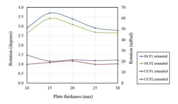
Figure 6.7: Rotation versus plate thickness for extended end-plate connection models
