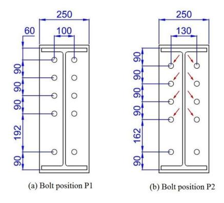
Figure 6.1: Position of bolt holes for the flush end-plate connection
