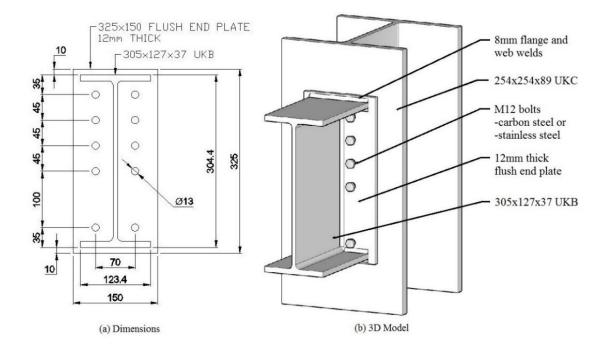
Figure 3.3: Flush end plate connection
