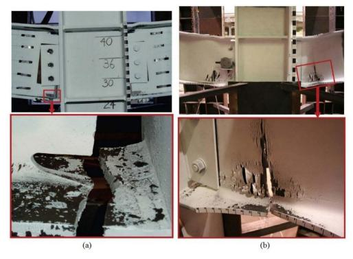
Figure 2.17: Failure mode of (a) WUF-B specimen and (b) RBS specimen (Lew et al. 2013)
