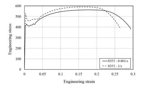
Figure 4.7: Engineering stress versus engineering strain
