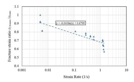
Figure 4.14: Fracture strain ratio  $\frac{\varepsilon_{f,dyn}}{\varepsilon_{f,stat}}$  versus strain rate for stainless steel bolts
