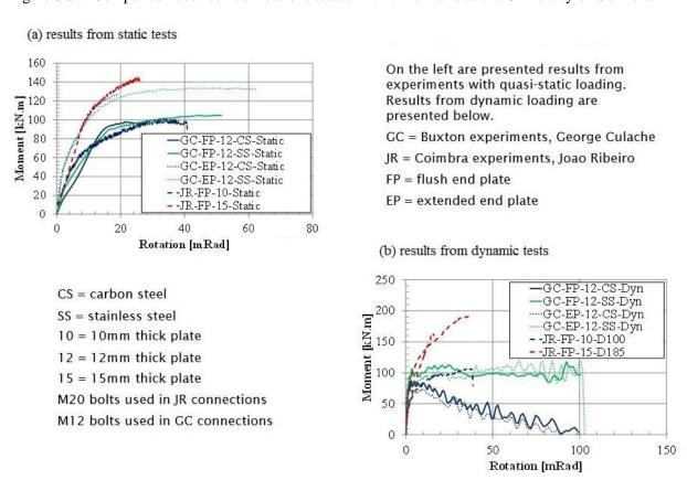
Figure 3.35: Comparison of moment versus rotation graphs
