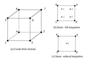
Figure 4.4: The continuum brick element (Simulia 2015b)
