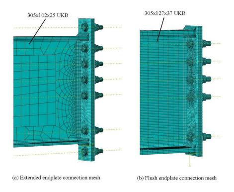
Figure 5.3: The two different types of model connections
