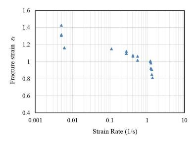
Figure 3.14: Fracture strain versus strain rate for stainless steel bolts
