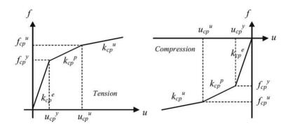
Figure 2.5: Force-displacement characteristic for components in tension and compression
