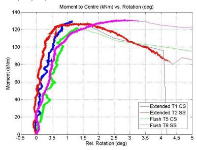
Figure B 15: Moment rotation graphs for tests T1, T2, T5, T6
