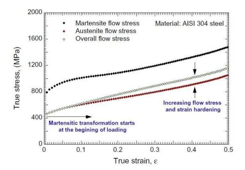
Figure 2.28: Evolution of martensite flow stress, austenite flow stress and homogenized flow stress as a function of strain for  $\dot{\varepsilon} = 100s^{-1}$  (Zaera et al. 2012)
