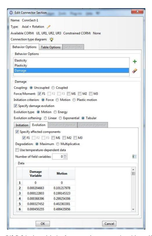
Figure C 12: Defining damage behaviour for connector elements representing stainless steel bolts
