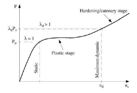
Figure 2.14: Characteristic nonlinear static response under proportional load ( $P = \lambda P_0$ ) (Izzuddin et al. 2008)
