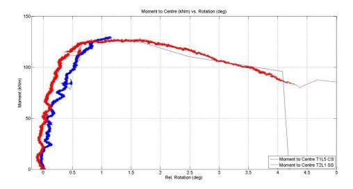
Figure B 9:T1, T2 - Moment to Centre (kNm) vs. Rotation (degrees)
