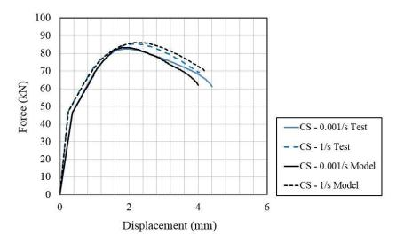
Figure 4.24: Comparison of force-displacement graphs for carbon steel bolts (test and FE predictions) for different strain rates (0.001 strain/s and 1 strain/s)
