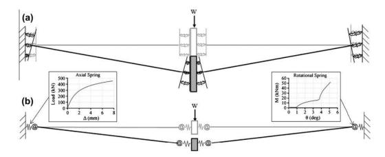
Figure 2.20: Column loss scenario using (a) component method and (b) rotational spring (Stoddart et al. 2013)
