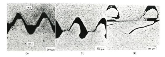
Figure 2.9: Examples of the deformation and damage from increasing pressures of (a) 25 MPa (b) 49 MPa (c) Thread stripping at impact energy of 120 J (Mouritz 1994)
