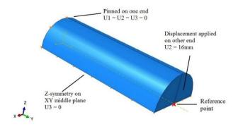
Figure 4.15: Model and boundary conditions
