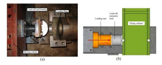
Figure 3.19: (a) Photo of load cell and loading ram and (b) illustration of force path through ram
