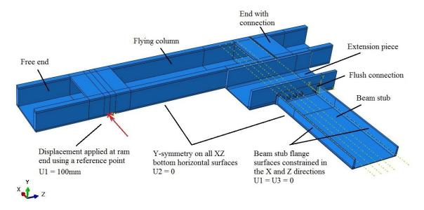
Figure 5.1: Geometry, model and boundary conditions of column-beam assembly
