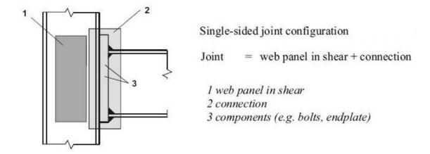
Figure 2.2: Parts of a beam-to-column joint configuration (CEN 2005)
