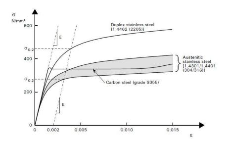
Figure 2.26: Example of difference in elastic-plastic transition for some carbon and stainless steels (Baddoo 2002)
