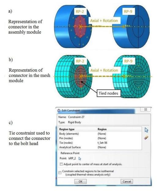
Figure 4.21: Representation of connector in the model and constraint needed to tie the connector to nodes of the bolt head and nut
