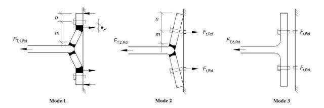
Figure 3.4: Possible T-stub failure modes, which are Mode 1, complete flange yielding, Mode 2, bolt failure with flange yielding, and Mode 3, bolt failure
