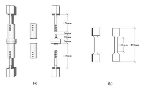
Figure 3.7: (a) Initial design of testing rig for bolts and (b) design of steel coupon
