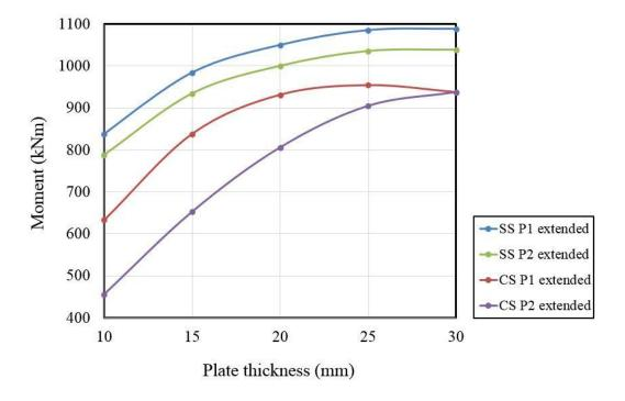
Figure 6.8: Moment versus plate thickness for extended end-plate connection models with stainless (SS) and carbon steel (CS) bolts
