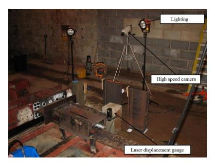
Figure 3.21: High speed camera and lighting set-up
