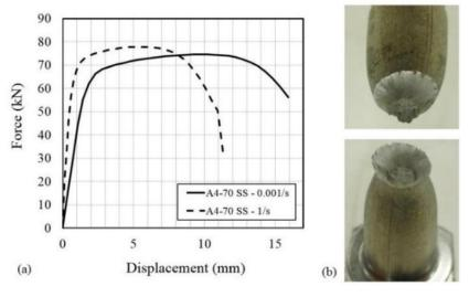
Figure 3.10: A4-70 stainless bolt, (a) force versus displacement and (b) fracture surface
