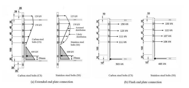
Figure 3.5: Force distributions for the calculated design moment capacity
