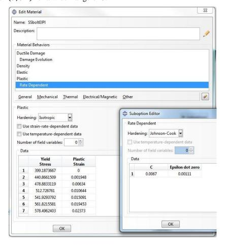
Figure C 6: Defining plastic behaviour for A4-70 stainless steel
