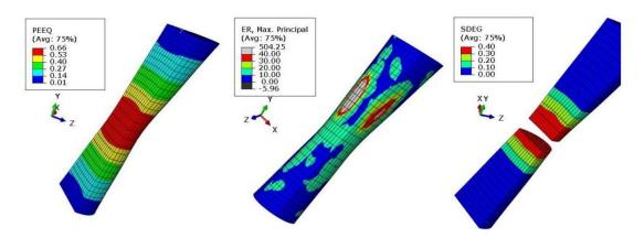
Figure 4.18: Contour plots of equivalent plastic strain (PEEQ) and strain rate (ER) at displacement of 11.05mm before fracture and scalar stiffness degradation (SDEG) after fracture
