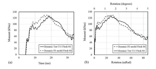
Figure 5.11: Moment versus rotation for extended end-plate model with stainless bolts
