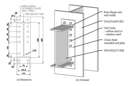
Figure 3.2: Extended end plate connection
