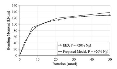
Figure 2.7: Proposed model by Del Savio et al. (2009) versus test EE3 by Lima et al. (2004)
