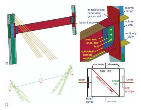
Figure 2.16: Steel assembly models with connection: (a) detailed; (b) reduced (Sadek et al. 2011)
