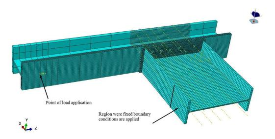
Figure 6.3: Finite element model mesh
