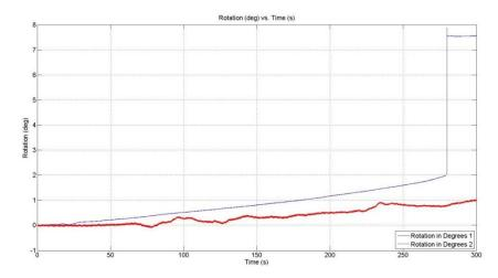
Figure B 10: T5 - Rotation (deg) vs. time (s) of "flying column" (blue) and angle supports (red)
