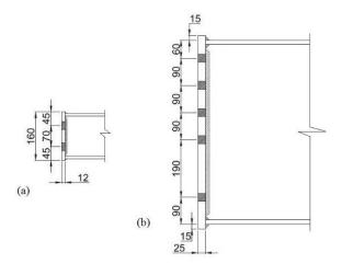
Figure 3.1: (a) Connection tested at University of Liege, (b) industry-standard connection
