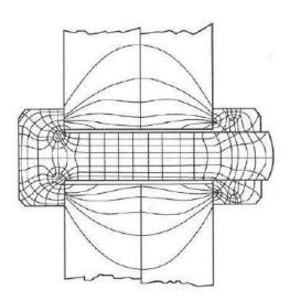
Figure 2.8: Lines of principal tension and compression in a bolt loaded in tension (Bickford 2007)
