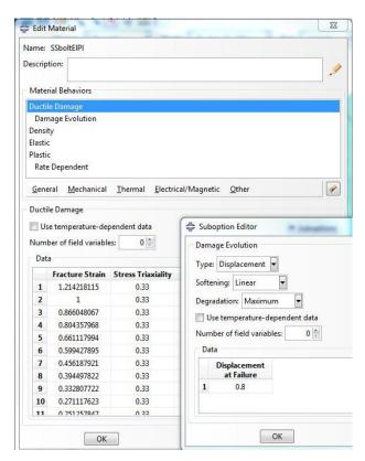
Figure C 8: Defining damage evolution for A4-70 stainless steel
