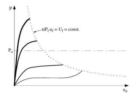
Figure 2.15: Different pseudo-static responses with identical energy absorption capacity (Izzuddin et al. 2008)
