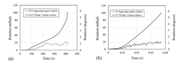
Figure 3.26: Rotation versus time for dynamic test T2A and T4
