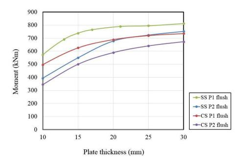
Figure 6.11: Moment versus plate thickness for flush end-plate connection models
