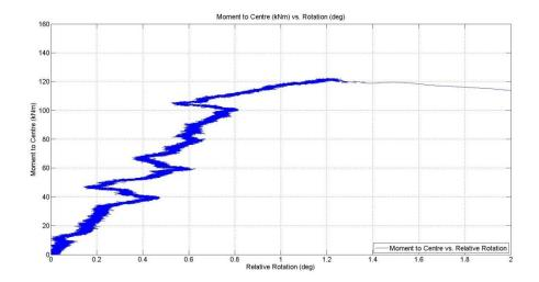
Figure B 11: T5 - Moment to Centre (kNm) vs. Net Rotation (degrees)
