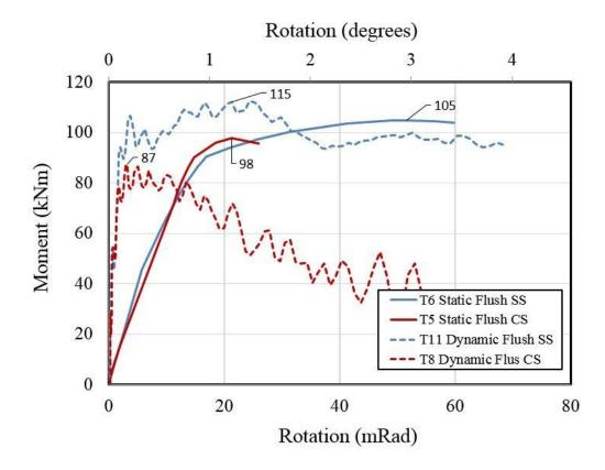
Figure 3.31: Moment versus rotation for static and dynamic flush plate tests
