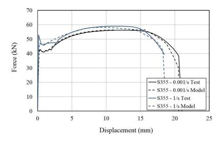
Figure 4.12: Force versus displacement result for tests and models at selected strain rates
