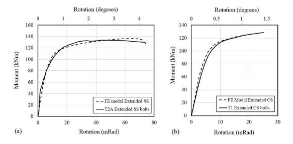
Figure 5.8: Moment versus rotation graphs for extended endplate connections tests and models
