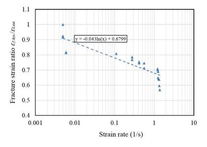
Figure 3.15: Fracture strain ratio  $\frac{\varepsilon_{f,dyn}}{\varepsilon_{f,stat}}$  versus strain rate for stainless steel bolt
