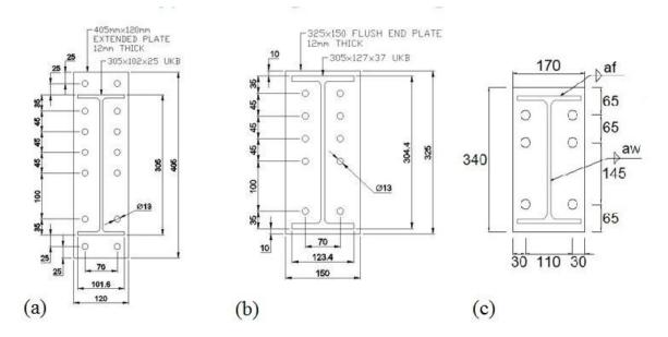
Figure 3.34: Comparison between connections tested in this work and at the University of Coimbra
