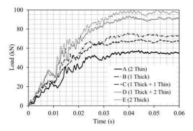
Figure 3.23: Diaphragm bursting trials (Stoddart 2012)
