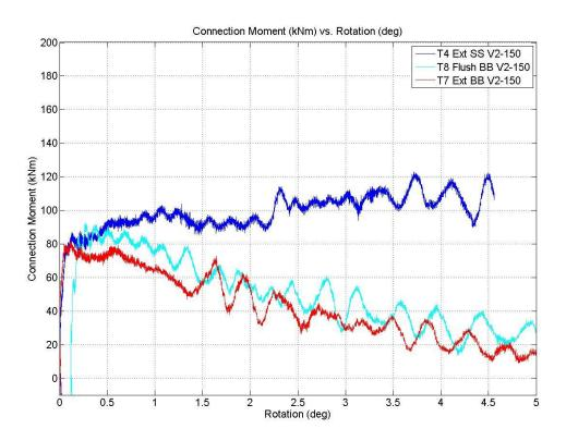
Figure B 55: T4, T7, T8 - Comparison of moment-rotation graphs from dynamic tests
