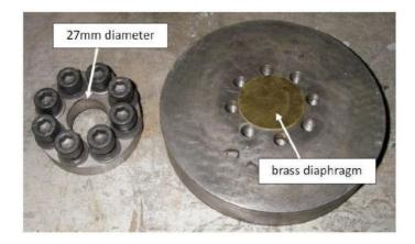
Figure 3.22: Diaphragm and cassette system (Stoddart 2012)
