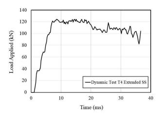
Figure 5.14: Applied load measured in the test and defined for the model
