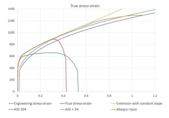
Figure D 1: Estimating true stress-strain curve for A4-70 using advanced Rusinek-Klepaczko (RK) material model for AISI 304 published by Rusinek et al. (2015)
