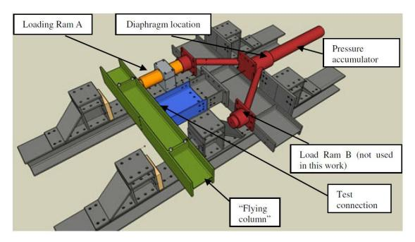
Figure 2.19: Testing rig used by Tyas et al. (2012)
