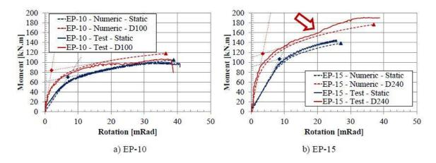
Figure 2.25: Comparison of the quasi-static and dynamic responses: a) EP-10; b) EP-15
