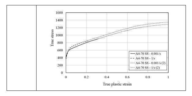
Figure C 6 shows some points from the set  $\{(\sigma, \varepsilon^{pl})\}$ , which is used to define the plastic behaviour. The plastic behaviour is defined by combining the set  $\{(\sigma, \varepsilon^{pl}, 0.0011s^{-1})\}$  with the Johnson-Cook test-calibrated C of 0.0067 and reference strain rate  $\dot{\varepsilon}_0$  of 0.0011 to allow prediction of  $(\sigma, \varepsilon^{pl})$  for a wider range of  $\dot{\varepsilon}$ .
