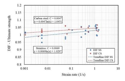
Figure 3.13: Dynamic increase factor (DIF) versus strain rate from bolt tests
