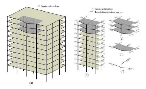
Figure 2.13: Building subjected to column loss and sub-structural levels for progressive collapse assessment (Izzuddin et al. 2008)
