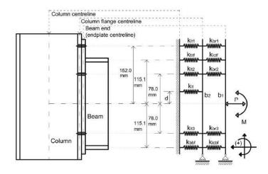
Figure 2.6: Proposed mechanical model for connection with tri-linear springs studied by Del Savio et al. (2009)
