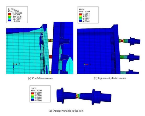
Figure 5.4: Contour plots of (a) Von Mises stresses, (b) plastic strains and (c) damage variable in the bolt for a connection rotation of 3.06 degrees when the applied moment reaches the maximum value of 108.5kNm
