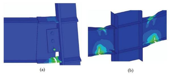
Figure 2.18: Failure mode from detailed model of (a) WUF-B connection and (b) RBS ("dog bone") connection (Sadek et al. 2013)
