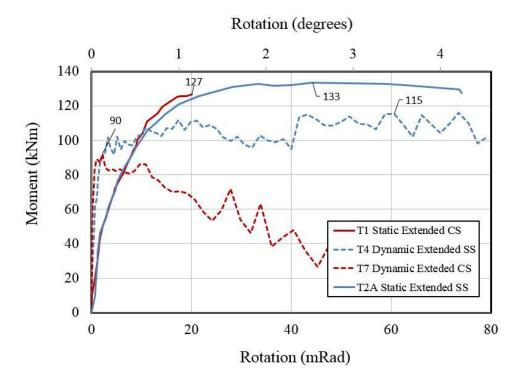
Figure 3.30: Moment versus rotation for static and dynamic extended plate tests
