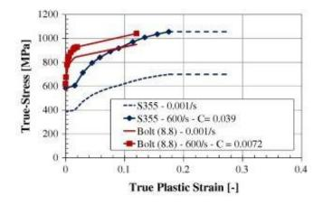
Figure 4.23: True stress true plastic strain curve (Ribeiro et al. 2016)
