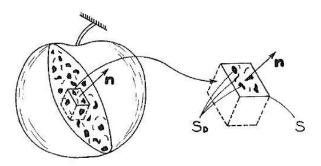
Figure 4.2: Damaged element (Lemaitre 1985)
