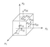
Figure 4.1: Unit cube in body subjected to tri-dimensional stress (Meyers & Chawla 2008)
