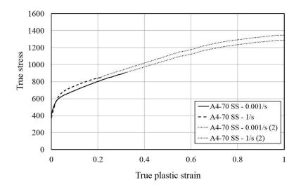
Figure 4.13: True stress versus true plastic strain curves at selected strain rates
