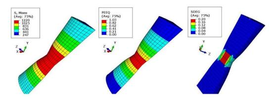
Figure 4.17: Contour plots of Von Mises stresses (S, Mises), equivalent plastic strain (PEEQ) and stiffness degradation (SDEG) at a total displacement of 14.10mm, step time 497.5s, before fracture
