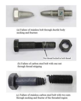
Figure 3.9: Failure mechanism for tested bolts
