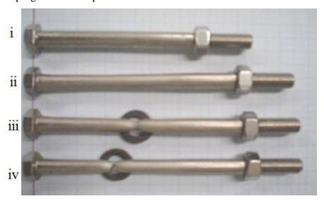
Figure 2.11: (i) Original stainless bolt (ii) bolt loaded at a low strain rate, (iii) medium strain rate and (iv) high strain rate (Munoz-Garcia et al. 2005)
