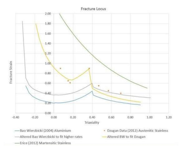
Figure D 2: Estimating fracture locus using functions found by Bao-Wierzibicki (2004) for aluminium and data points for stainless steel published by Dzugan et al. (2012)
