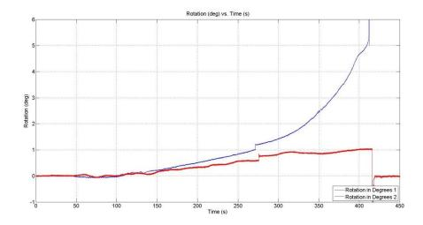
Figure B 7:T2 - Rotation (deg) vs. time (s) of "flying column" (blue) and angle supports (red)
