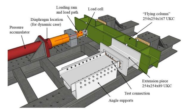
Figure 3.18: 3D model of testing rig used for testing of designed moment connections from low  $(0.001 \text{ s}^{-1})$  to high strain rates (up to  $100 \text{ s}^{-1}$ )
