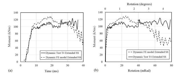
Figure 5.16: Moment versus rotation for extended end-plate model with stainless steel bolts
