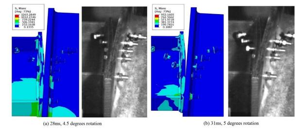
Figure 5.13: 3<sup>rd</sup> and 4<sup>th</sup> bolts fail at 28ms and 31ms, predicted and experimental results
