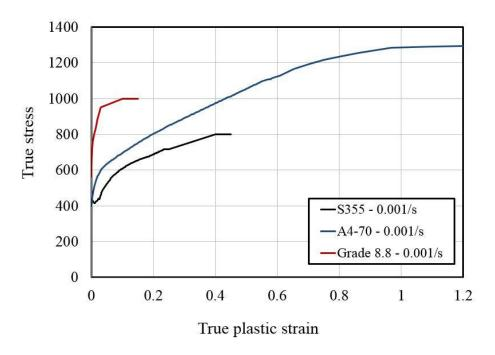
Figure 3.17: True stress versus true plastic strain for different materials
