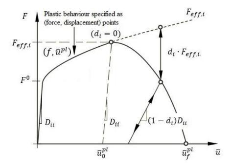
Figure 4.6: Force-displacement curve with progressive damage necessary for the definition of the behaviour of the connector element (Simulia 2015b)
