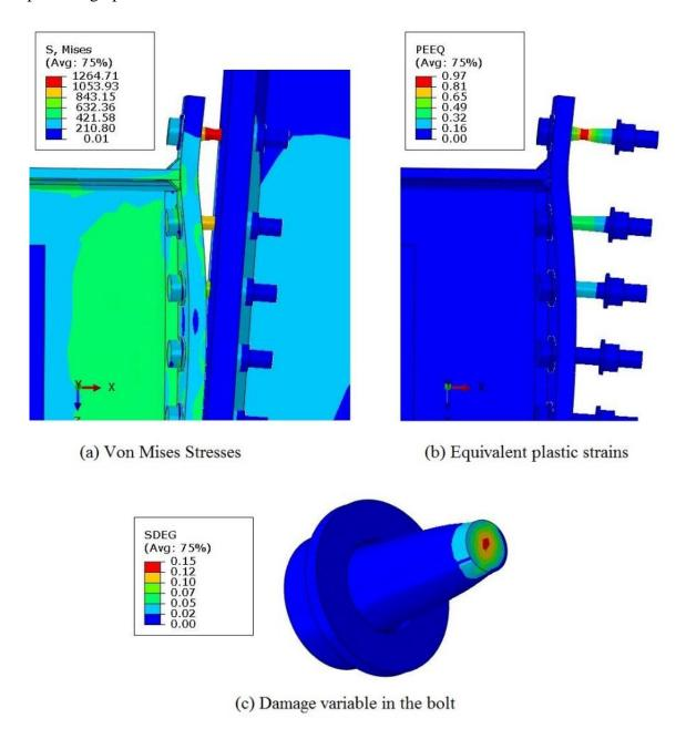
Figure 5.6: Contour plots of (a) Von Mises stresses, (b) plastic strains and (c) damage variable in the bolt for a connection rotation of 4.12 degrees when the moment reaches the value of 133kNm
