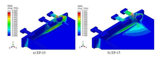
Figure 2.24: Dynamic numerical models failure – bolt rupture
