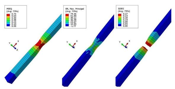
Figure 4.11: Contour plots of equivalent plastic strain (PEEQ) and strain rate (ER) at displacement of 18.12mm before fracture and scalar stiffness degradation (SDEG) after fracture
