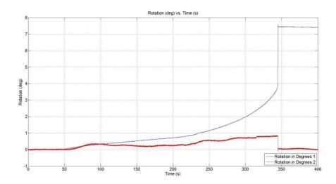
Figure B 12: T6 - Rotation (deg) vs. time (s) of "flying column" (blue) and angle supports (red)
