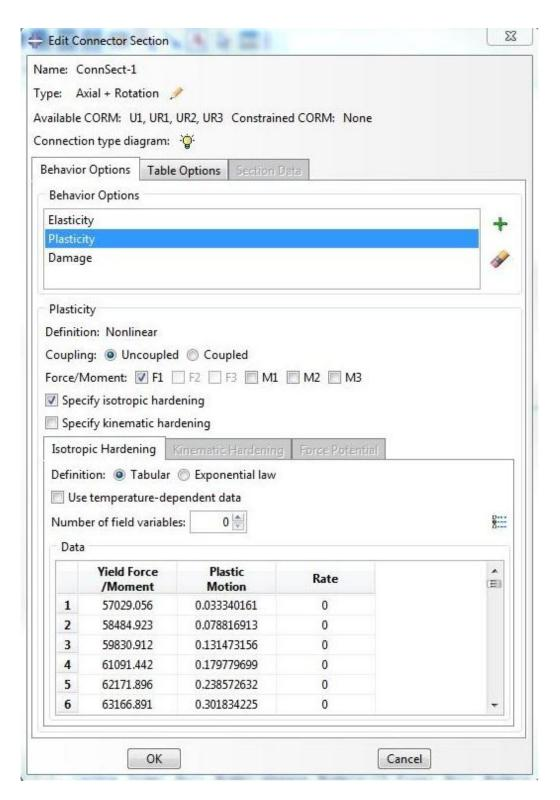
Figure C 11: Defining plastic behaviour for connector elements representing stainless steel bolts
