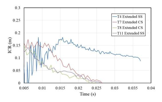
Figure 3.32: ICR vs time for dynamic tests, note changes are small in comparison to lever arm
