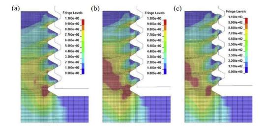
Figure 2.12: Stress distribution in a bolt-nut connection representing maximum principal stress during (a) elastic behaviour, (b) at maximum force, and (c) at beginning of failure (Fransplass et al.
