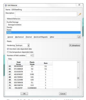
Figure C 2: Defining plastic behaviour of S355 steel
