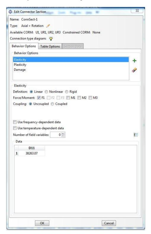
Figure C 10: Defining elastic behaviour for connector elements representing stainless steel bolts
