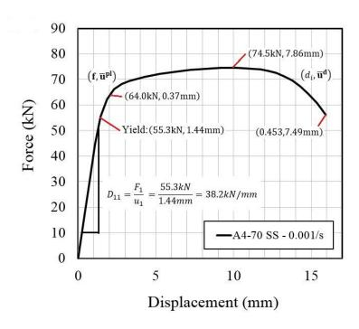
Figure 4.20: Graph and data defining connector behaviour
