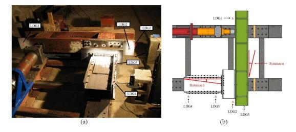
Figure 3.20: Displacement measurement locations illustrated on (a) photo of rig and (b) 3D model
