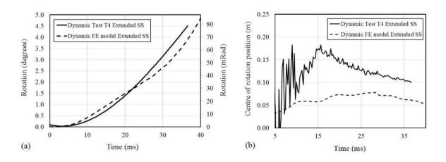
Figure 5.15: (a) Rotation versus time and (b) ICR versus time, note changes are small in comparison to lever arm
