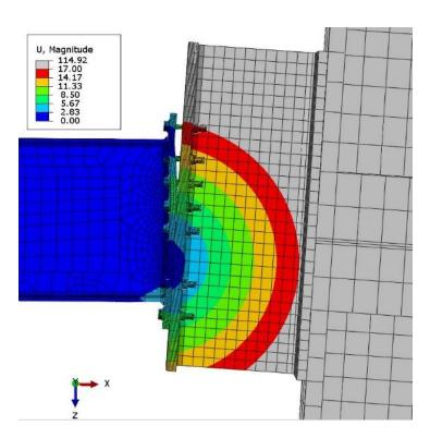
Figure 5.5: Contour plot for total displacements, mainly X direction, for the connection close to failure
