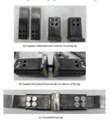
Figure 3.8: Bolt testing rig used for testing bolts from low  $(0.001 \text{ s}^{-1})$  to medium strain rates  $(1 \text{ s}^{-1})$
