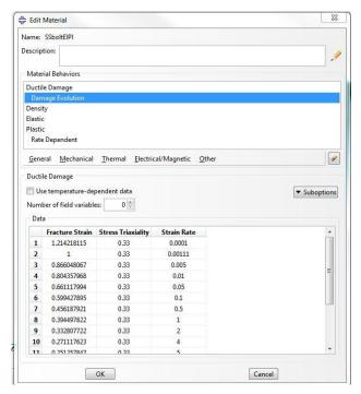
Figure C 7: Defining fracture strain for A4-70 stainless steel
