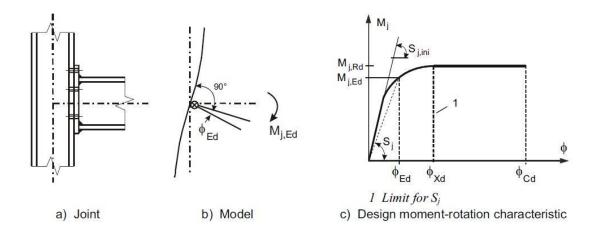
Figure 2.4: Design moment-rotation characteristic for a joint (CEN 2005)
