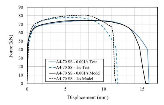
Figure 4.22: Comparison of force-displacement graphs from stainless steel bolt tests and finite element models at two selected stain rates (0.001 strain/s and 1 strain/s)
