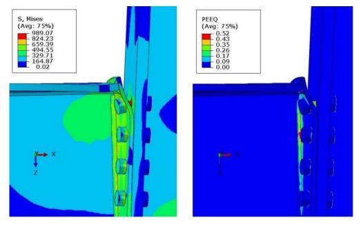
(a) equivalent stresses and plastic strains for 10mm thick flush end-plate
