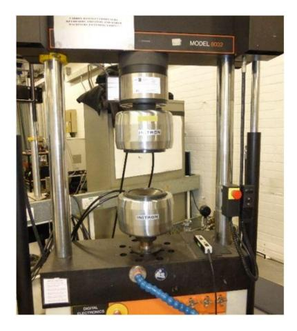
Figure 3.6: INSTRON 8032 testing apparatus
