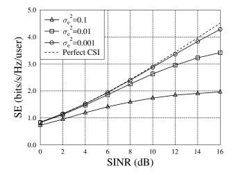
Fig. 6: SE versus the target SINR for CTSN systems under imperfect CSI, where Gaussian signalling waveforms are assumed. The satellite using  $N_{\rm S} = 8$  TAs supports  $G_{\rm S} = 4$ multicast groups. Two terrestrial BSs with  $N_{\rm B} = 8$  provide multicast services to  $G_{\rm B} = 8$  multicast groups. The variance of channel errors is  $\sigma_e^2 = 0.001, 0.01, \text{ and } 0.1$ .
