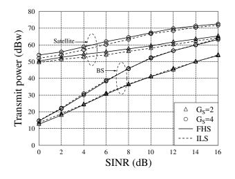
Fig. 4: Transmit power versus the target SINR for CTSN systems under perfect CSI, where Gaussian signalling waveforms are assumed. The satellite using  $N_{\rm S} = 4$  TAs supports  $G_{\rm S}$  multicast groups. Two terrestrial BSs employing  $N_{\rm B} = 4$  provide multicast services to  $G_{\rm B} = 4$  multicast groups.
