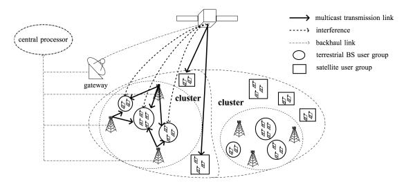
Fig. 1: Illustration of a multimedia multicast scenario in a cloud-based terrestrial-satellite network (CTSN), where the same frequency band is shared by users within a given cluster.
