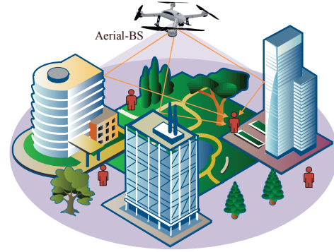
Fig. 1. The air-ground mmWave channels between the UAV aerial-BS and UD exhibit sparsity in both angle-domain and delay-domain due to the limited significant scatterers [25], [26].
