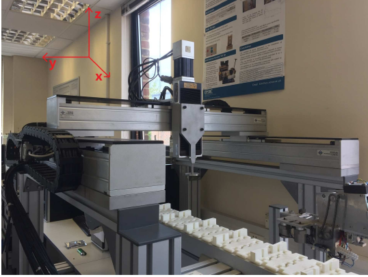
Figure 2: Multi-axis gantry robot test platform.
