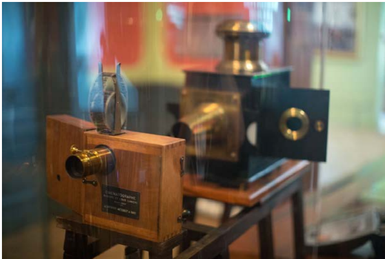
Still 4.4: The dual projector and camera, Cinématographe Lumière, as displayed at the Institut Lumière, Lyon. [Source: Wikimedia Commons (Victorgrigos, 2014, CC BY-SA-4.0)].
