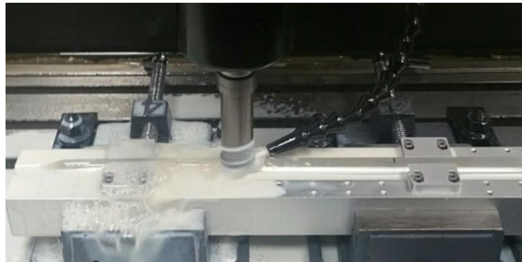
Figure 62: Milling of preform on customized milling stage with Standard Series 10 Rotary Knee mill from SONIC-MILL.
