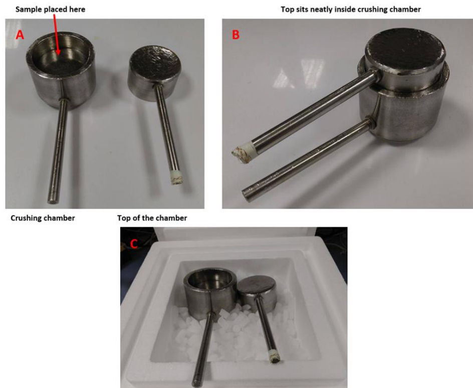
Figure 2-10 Tissue crushing equipment A) Crushing chamber. B) Crushing chamber assembled for use. C) Crushing chamber is cooled on dry ice prior to use.
