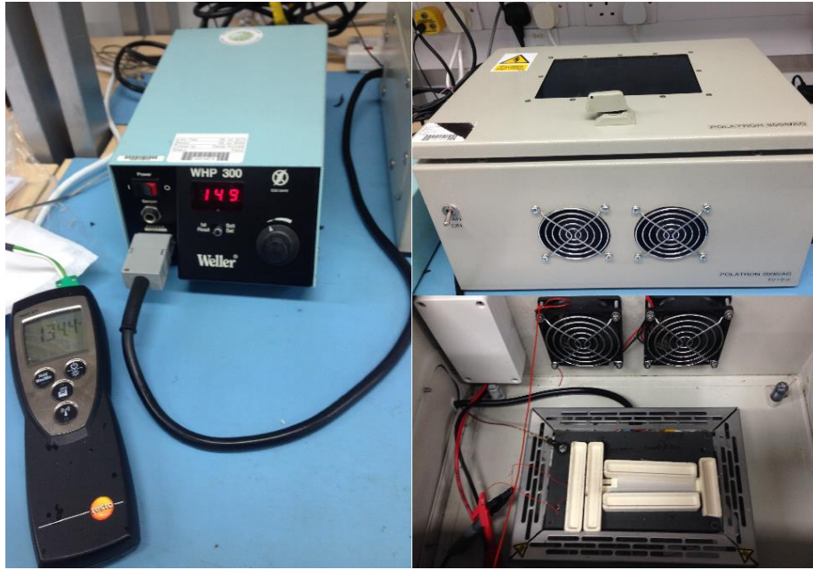
Figure 106. Polatron 2006. Left: thermocouple, top right: polarisation box, bottom right: hot plate with a sample.
