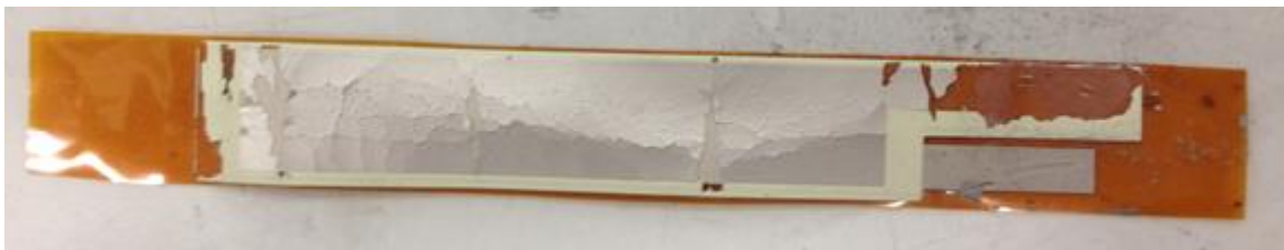
Figure 111. Catastrophic damage to the piezoelectric film.
