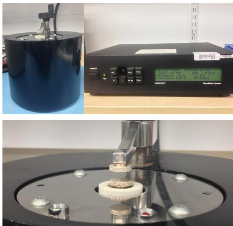
Figure 107. Top: PIEZOTEST PM300 set. Bottom: Sample clamping area.
