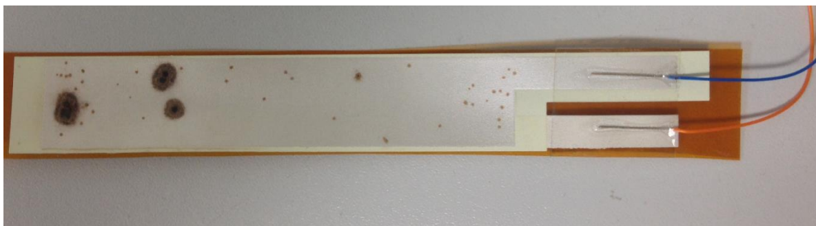
Figure 108. Piezoelectric film with small and large pinholes.
