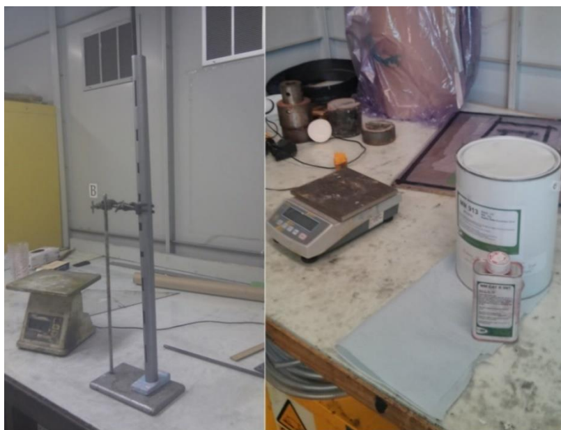
Figure 22. Casting apparatus and the two-part silicone compound.
