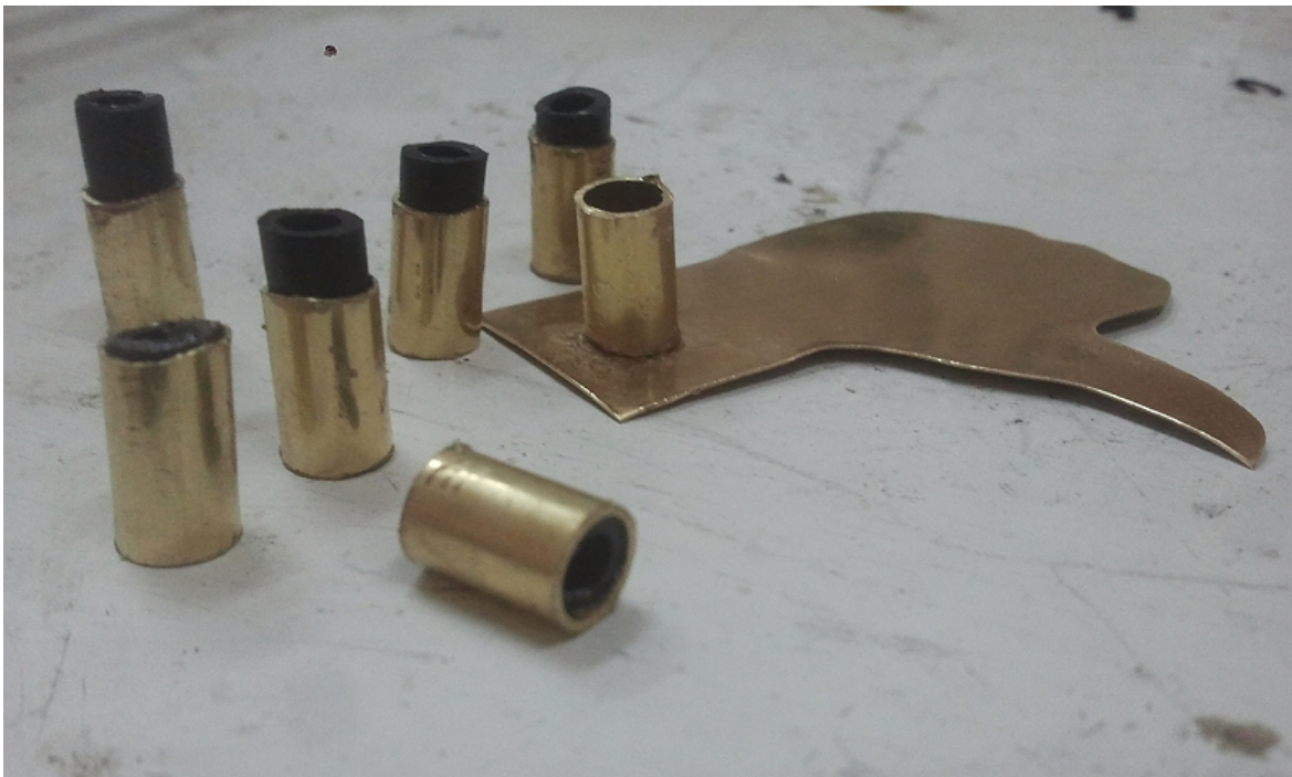
Figure 28 Detail of one hand and the cylinder that holds it to the rotating axis. Inside the cylinder, a piece of rubber ensures the transmission of the rotation.
