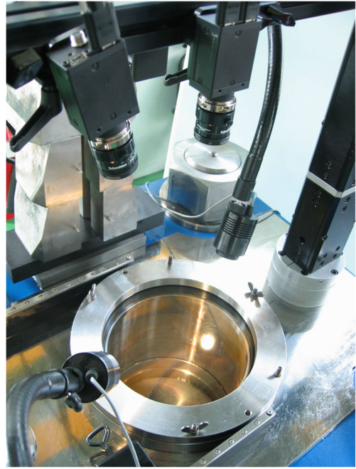
Fig. 7 View of the bulge test experimental set-up
