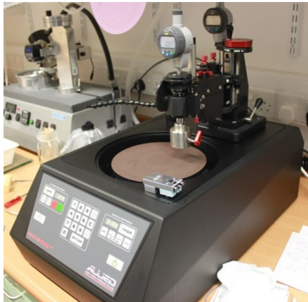
Figure 2.11: OptiPrep (Allied Technology) polishing system used for much of the polishing work.
