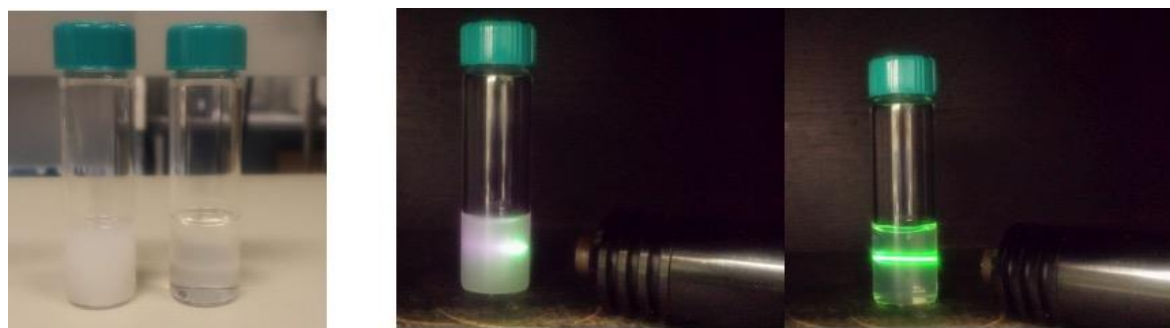
Figure 63. From left to right. Digital images of \beta -NaYF 4 :Yb 3+ (20%), Er 3+ (2%) UCNPs dispersed in hexane under ambient light and under a 980 nm laser pointer before and after annealing at 240 °C for 1.5 hour.
