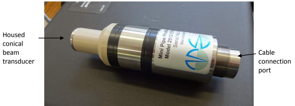
Figure 3.4 Mini Pipe Profiling Sonar Device (Model 2512).
