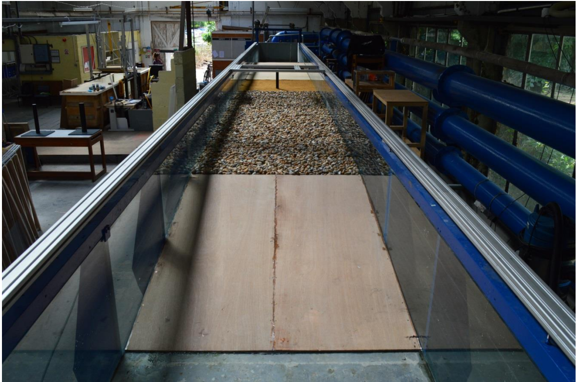
Figure 3.2 Constructed false flooring viewed from upstream.
