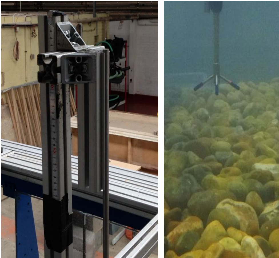
Figure 3.10 Acoustic Doppler Velocimeter support (left) and submerged receiver head (right).
