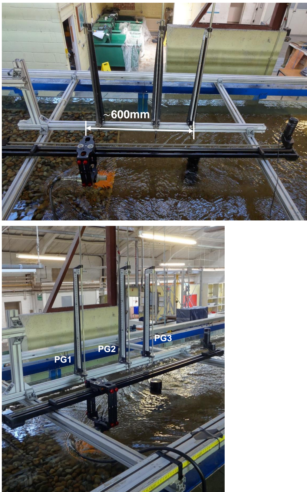
Figure 3.13 Overview of apparatus set-up. Idle sonar is positioned upstream of the test area. PG1, PG2 and PG3 represent point-gauges installed to check the elevation of the sonar outputs.
