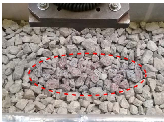
Figure 5. Marked grains placed in the ballast bed before being covered
