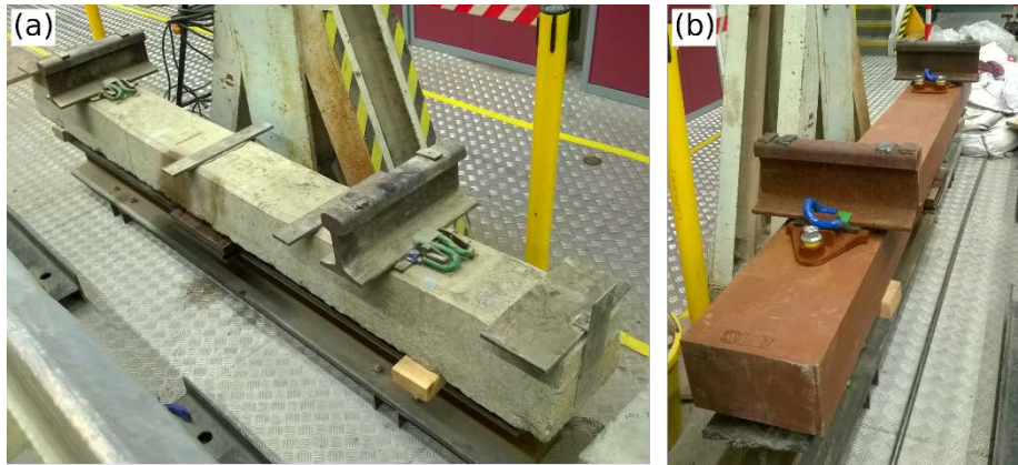
Figure 2. Sleepers tested: (a) steel prestressed concrete (b) composite
