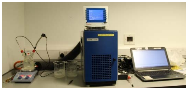
Figure 1. The water bath in the middle provides the temperature control of the magnetically stirred crystallising vessel on the left via circulating water to the jacket. The turbidity and temperature probes in the vessel send data to the computer on the right.
