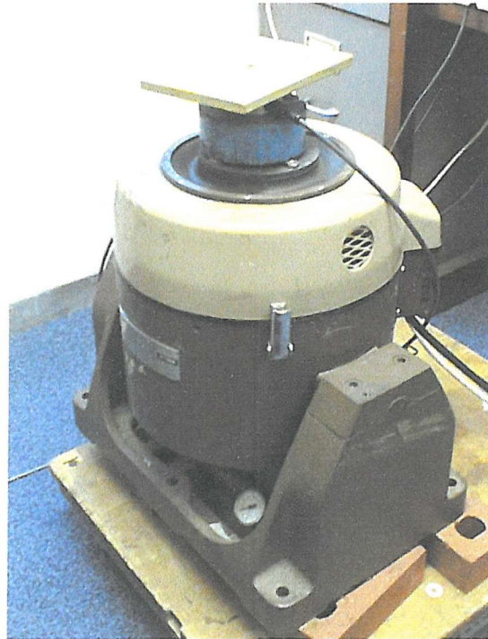
Figure 3-5 Exterior view of the VP 30 vibrator with a force cell and a wooden plate at the top.
