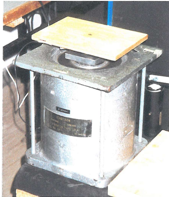
Figure 3-4 Exterior view of the VP 4 vibrator with a force cell and a wooden plate at the top.
