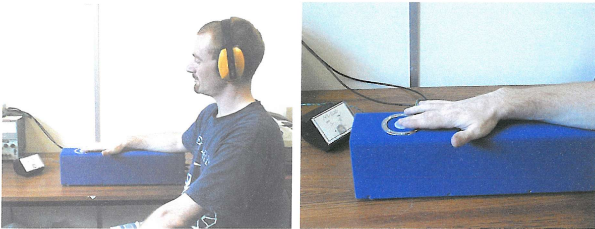
Figure 4-1 Experimental view of vibrotactile threshold measurement using a HVLab Tactile Vibrometer.
