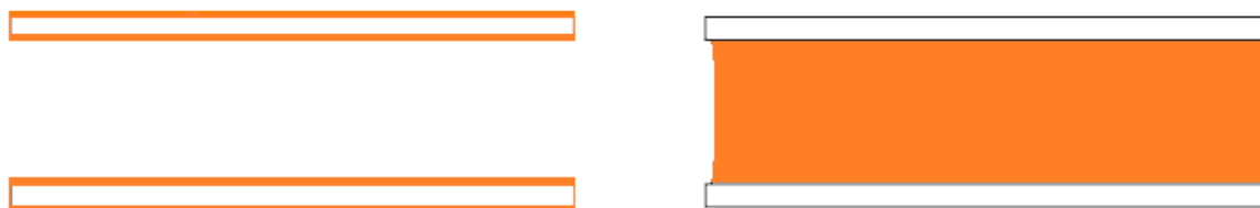
Figure 4.12. Schematic representation of a nanotube cross section with a monolayer of a selected molecule adsorbed on the surface (left) and encapsulated in the inner hollow nanostructure (right).
