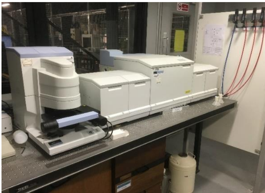
Figure 3.19: Photograph of the Fourier transform infrared spectroscopy instrument.
