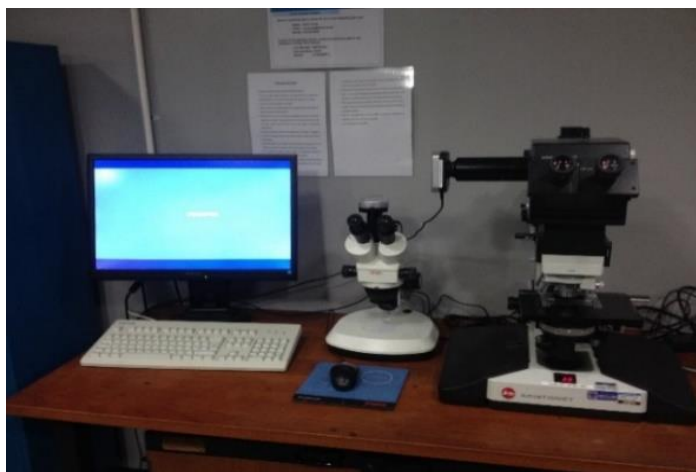
Figure 3.10: Photograph of the optical microscopy instrument.
