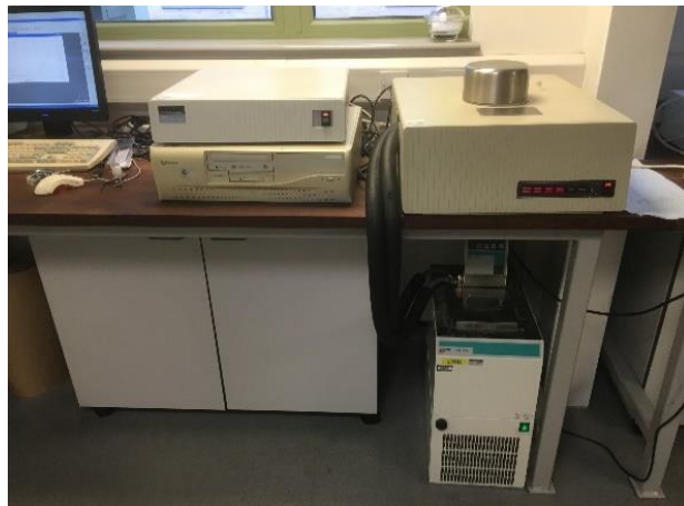
Figure 3.15: Photograph of the differential scanning calorimetry instrument.
