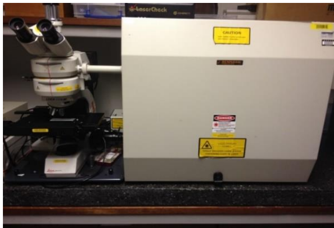
Figure 3.23: Photograph of the Raman spectroscopy instrument.
