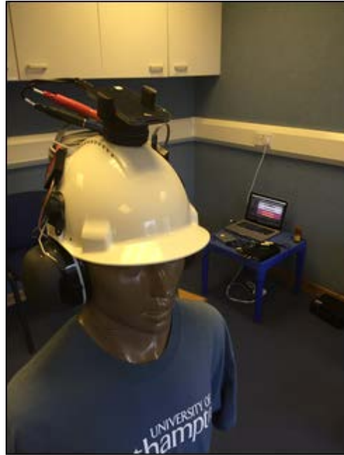
Figure 8.4 - Real-time hearing loss simulation device worn by the KEMAR mannequin.
