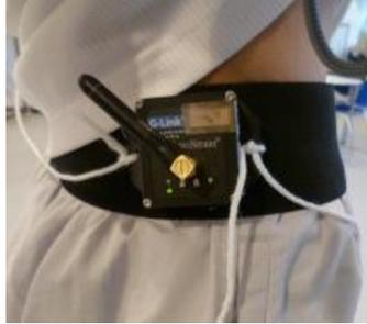
Figure 3.5 The wireless tri-axial accelerometer mounted on the hip [104]
