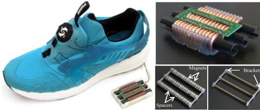
Figure 2.9. The electromagnetic energy harvester for shoe integration by Ylli *et al* [48].
