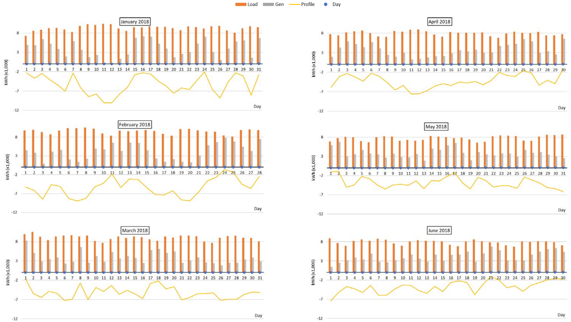
Figure 19: January - June 2018 Load, Generation and Profile
