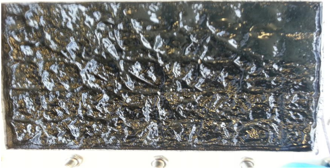
Figure 5-14: Photo of cake layer formed during continuous operational flux of around 30 \text{ L m}^{-2} \text{ h}^{-1} at the end of the continuous operation cycle prior to cleaning with tap water.
