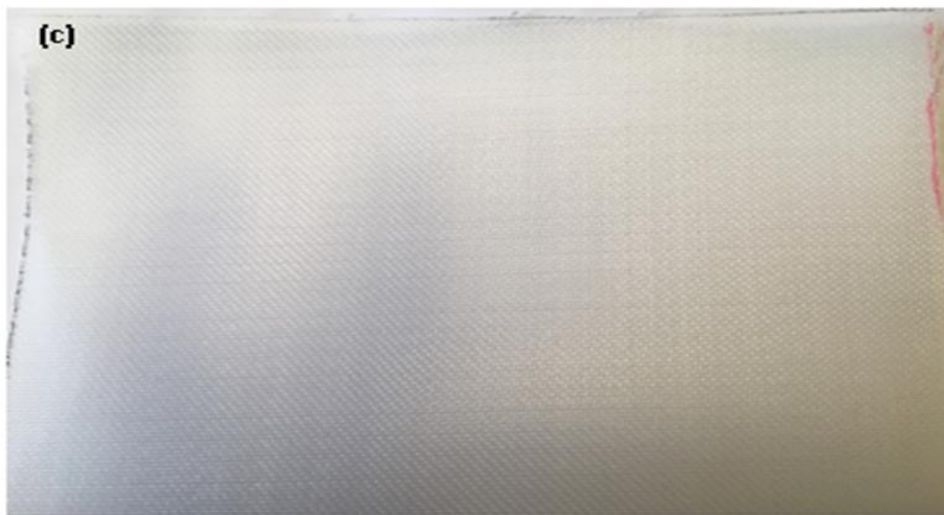
Figure 4-1 : Photos of support materials used (a) nylon mesh (b) woven polypropylene (c) non-woven polypropylene
