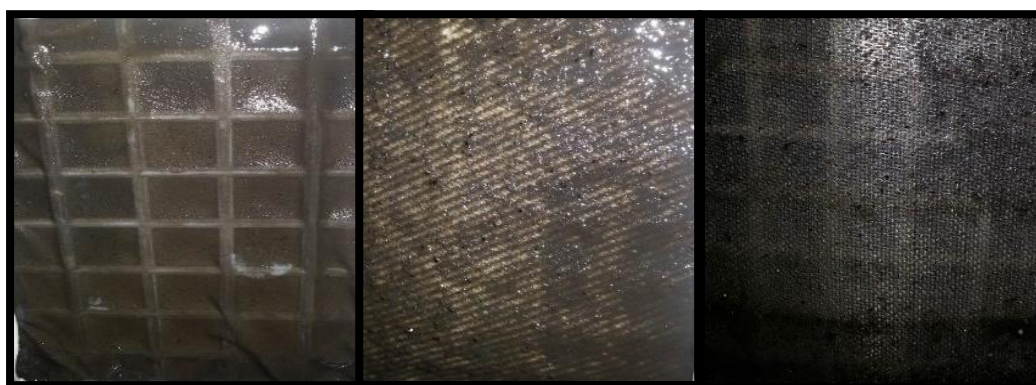
Figure 4-8: Images of support materials showing deposition when subjected to 5 TSS g L -1 1 a) nylon b) woven polypropylene c) non-woven polypropylene
