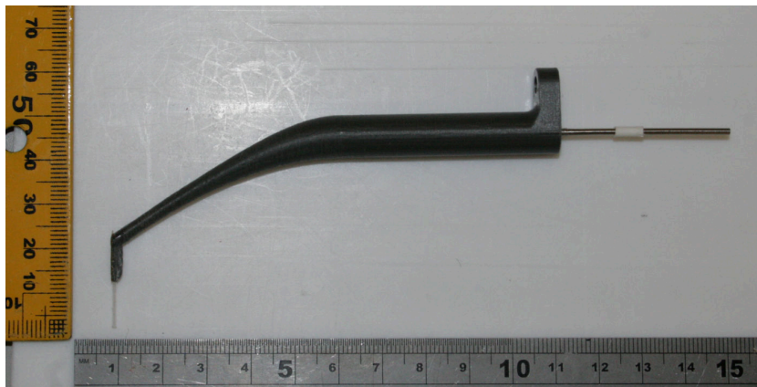
Figure 4.10: Capillary total pressure probe utilised in the study.
