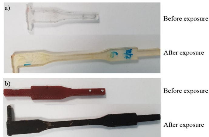
Figure 8.2: Decolourisation of a) brittle (Araldite 2020) and b) ductile adhesive (Araldite 2047-1) after exposure.
