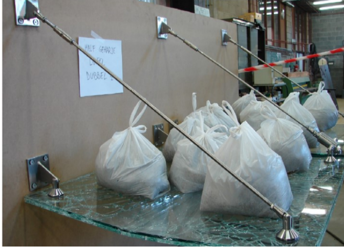
Figure 2.15: Adhesively bonded point fixings for a suspended canopy test [90].
