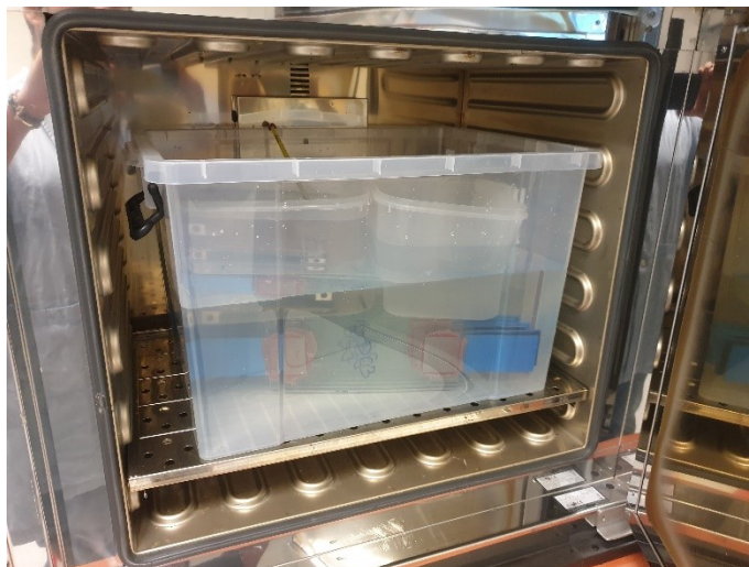
Figure 8.1: Exposure of glass/steel double lap shear adhesive joints.
