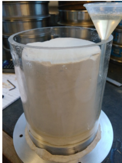
Figure 4.24. Filling of specimen-confinement pipe gap with epoxy resin using a small funnel.
