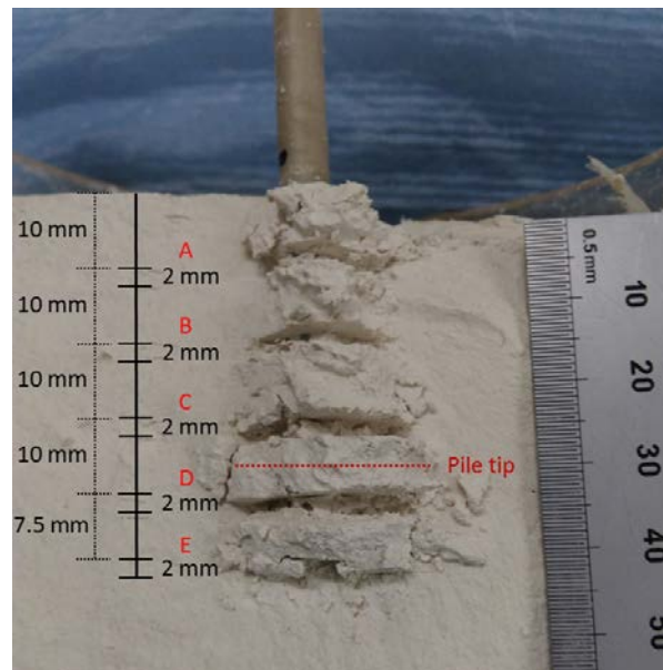
Figure 4.37. Detail of exhumation of CT02 and extraction of annulus samples.
