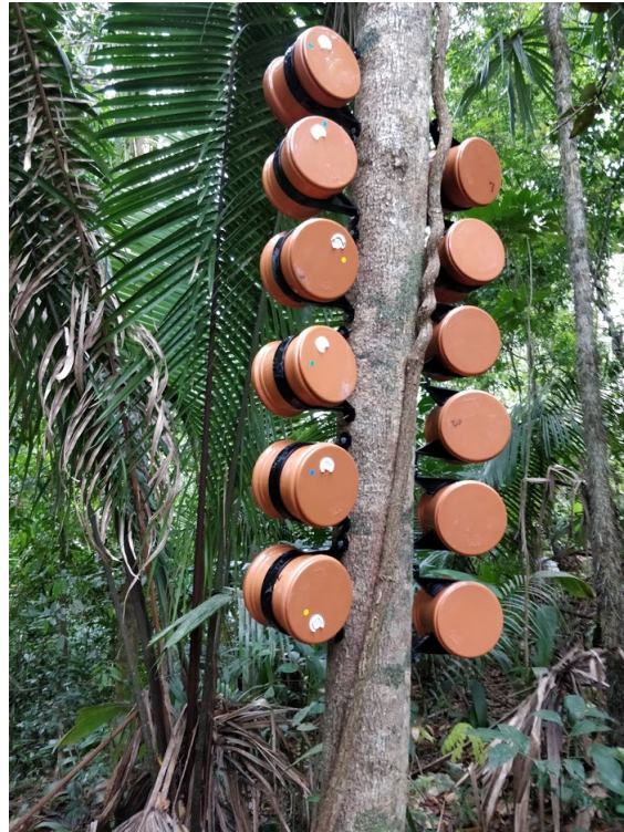
FIGURE 7.2: Twelve AudioMoth devices deployed in cases constructed from plastic piping, prepared for a series of field tests aiming to calculate the accuracy of the device and algorithm at various distances.
