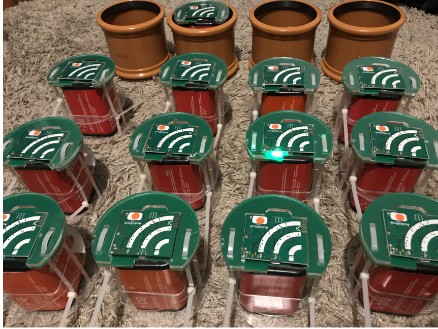
FIGURE 5.7: AudioMoths equipped with 6 V batteries, ready for deployment in Belize. Each unit consisted of four pieces of laser-cut plastic, a battery and an AudioMoth, held together using two cable-ties. These units were protected by capped plastic pipes and acoustic membrane stickers.
