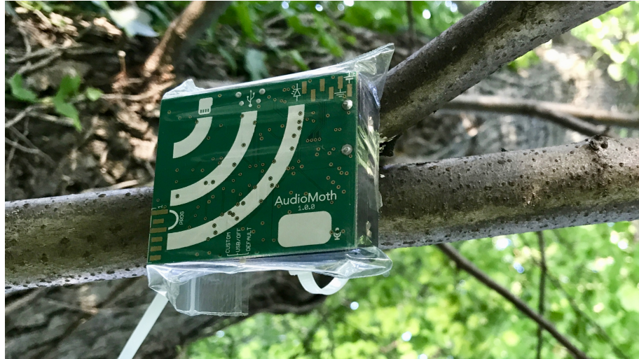
FIGURE 3.3: An AudioMoth deployed in a grip-sealed bag with a silica gel sachet to prevent the build-up of moisture, secured to a branch using a cable-tie.
