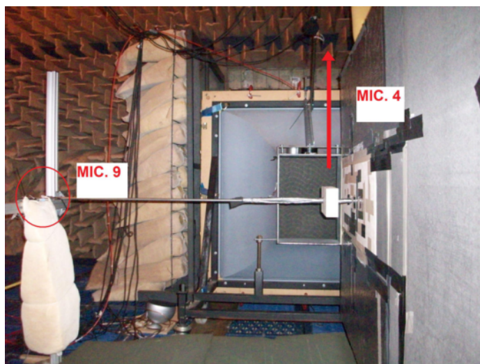
Figure 2.15: Experimental set-up used for the noise tests of simple geometries including the cube ( Latorre Iglesias, 2015 )
