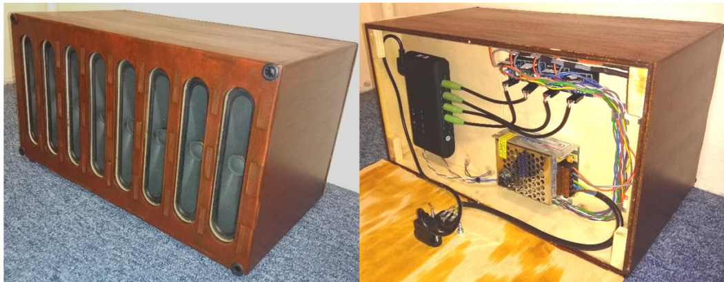
Figure 5: 8-Channel loudspeaker array. Left: Front view; Right: Rear view with back panel removed.
