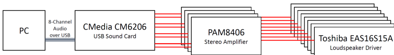
Figure 3: Loudspeaker array system block diagram.
