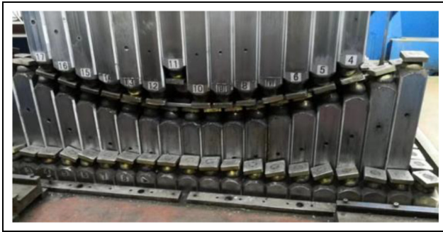
Figure 15. Plate is compacted by dies.
