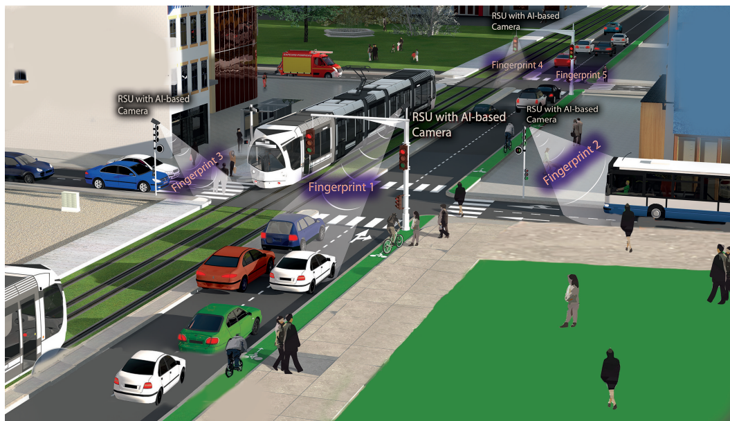
Figure 7.5: Fingerprint based beam-alignment for fast initial access.
