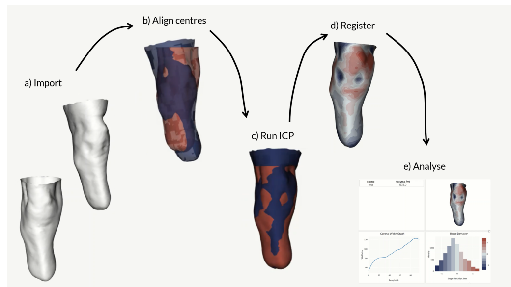
Figure 1: A graphical summary of a typical ampscan process. a) Importing a pair of scans, b) Automatically snap centres, c) Align using ICP algorithm, d) Register and visualise shape deviation and e) Automatically analyse the registered scan
