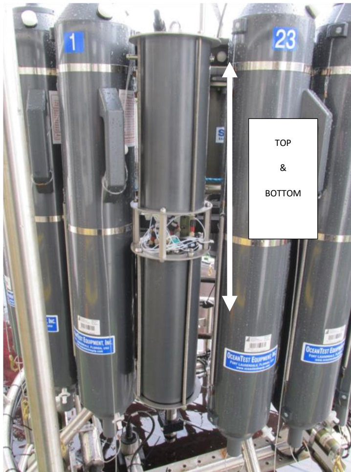
Figure 2.5: A LoC nutrient sensor within a custom frame mounted on a CTD rosette system in place of a single Niskin bottle. The LoC sensor and battery are located within the bottom grey section, while the blood bags for the reagents, nitrate standard and waste are located in the top section. The 0.45\ \mu\text{m} MILLEX-HP filter unit can be seen located between both the top and bottom sections.
