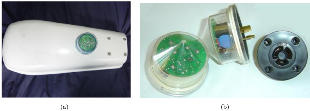
Figure 2.7: (a) A streetlight fitted with a photo electric control unit (PECU); (b) Typical PECUs (reproduced from [99]).
